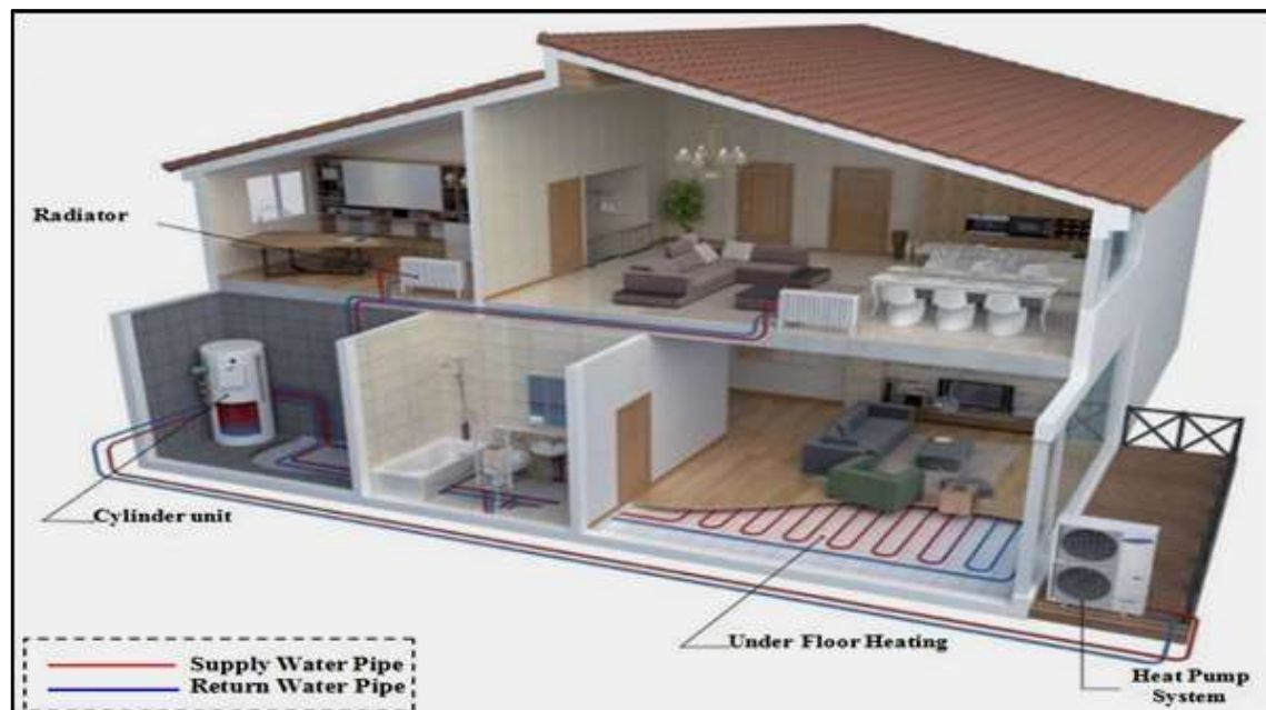
Figure 5: Description of the Elements of Heat Pump Water Heater System
