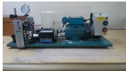
Figure 16: Alternative bending fatigue machine.
