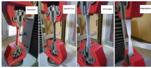
Figure 6: Specimens under tensile test.
