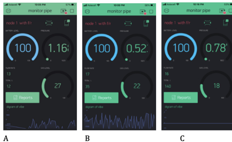
Figure 14: A. sensor measurements without event on the pipe. B. a lake five meters away from the beginning of the pipe. C. a lake fifteen meters away from the beginning of the pipe.
