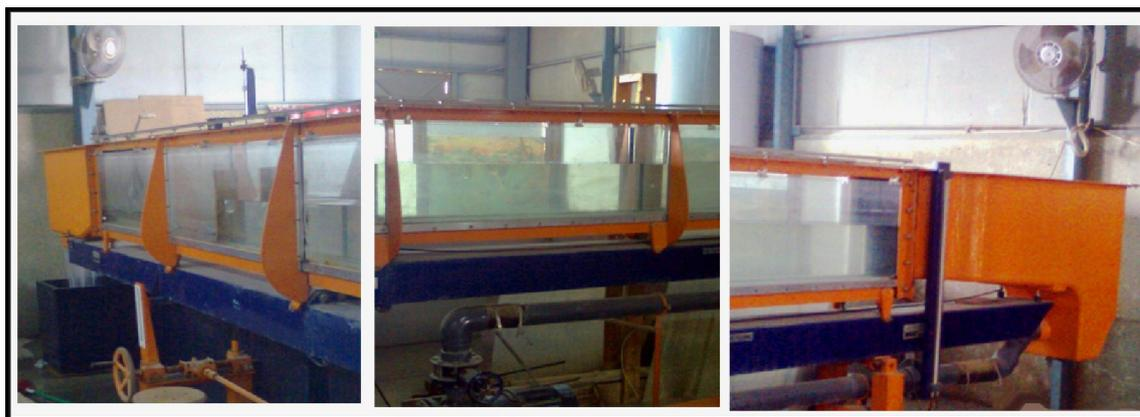
**Figure(4): S6-Tilting flume front and side views**
