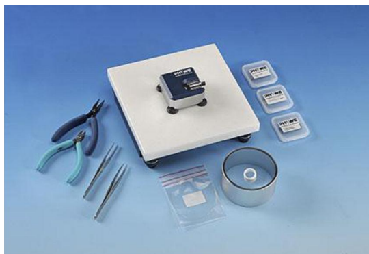
Fig. (1) Components of the PHYWE Compact STM.
