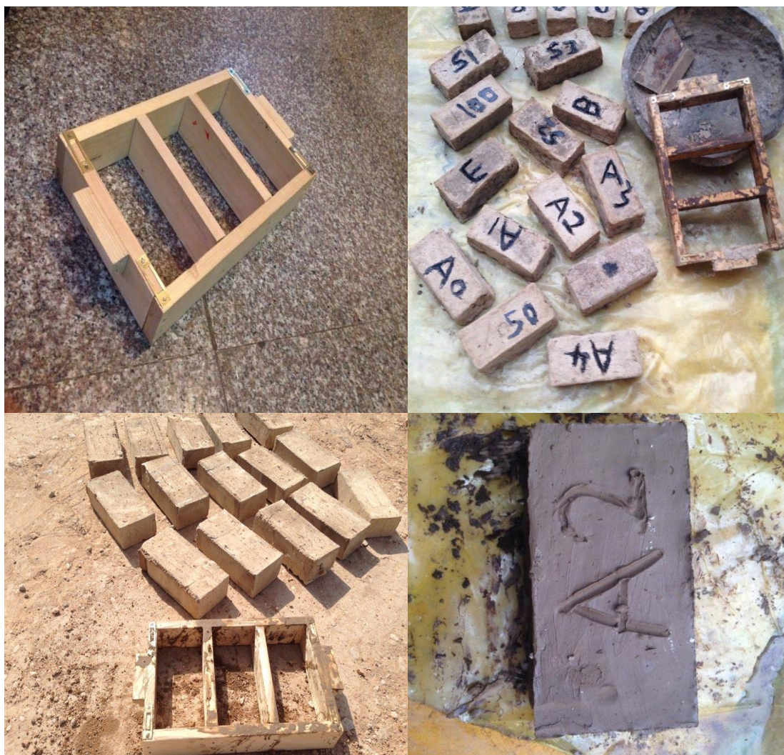
Plate(1): Mold and Specimens of Clay Brick Made with Adding of (marble dust)
