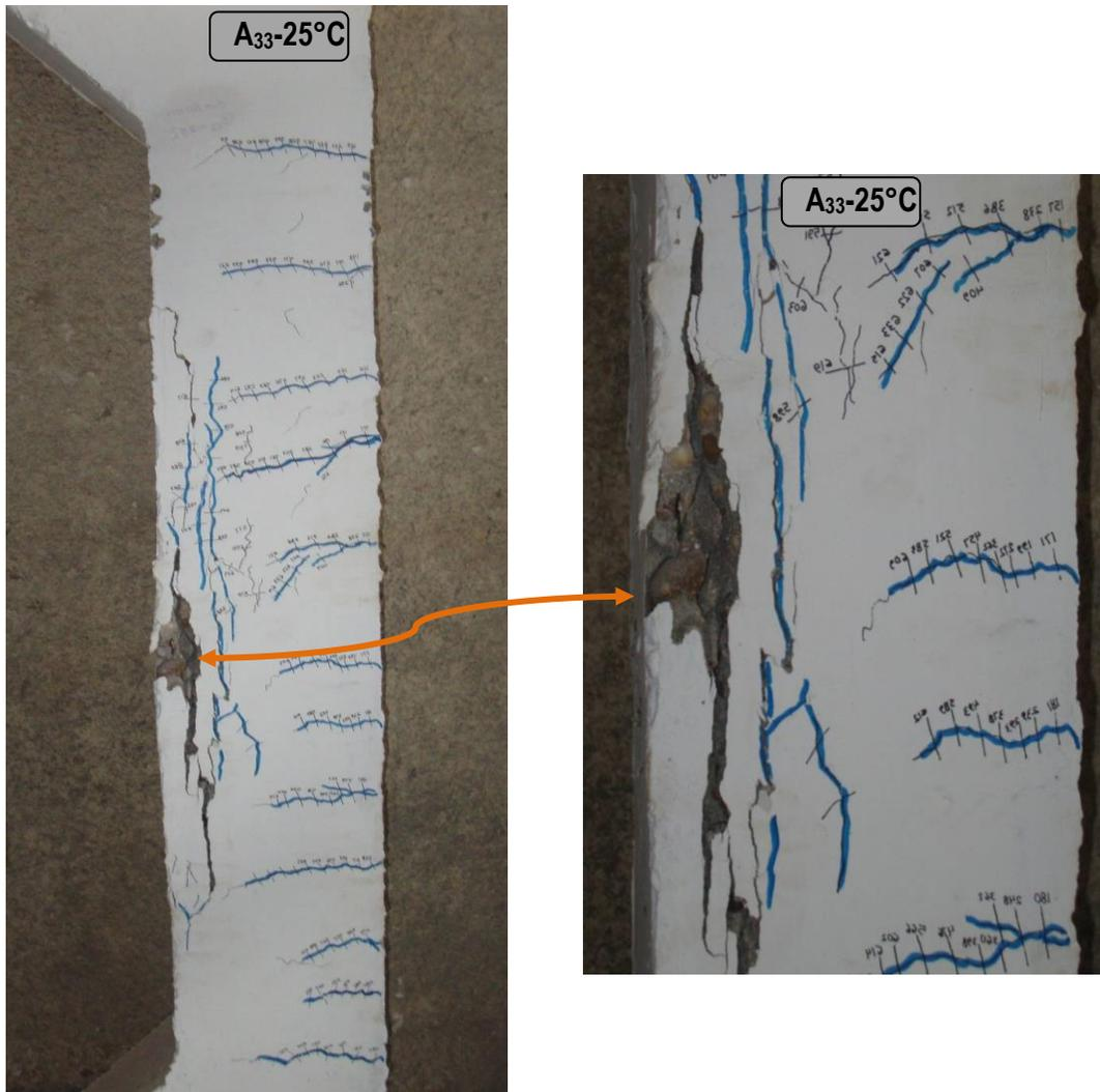
Plate (5): Typical crack pattern of series A column specimens with different tie spacing and subjected to eccentric loading ( $e=80\text{mm}$ ) at failure.
