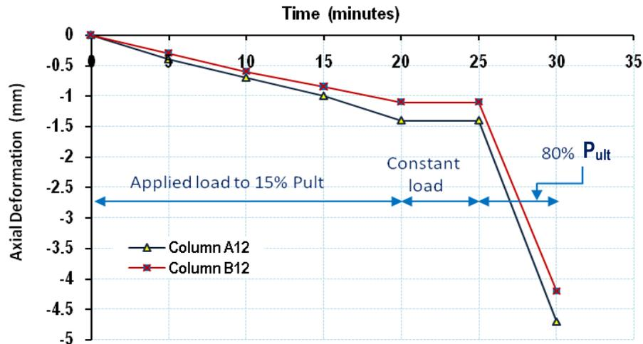
Figure (8): Axial deformation versus time curve at centerline of column specimens A12 and B12 without burning, 25 °C.
