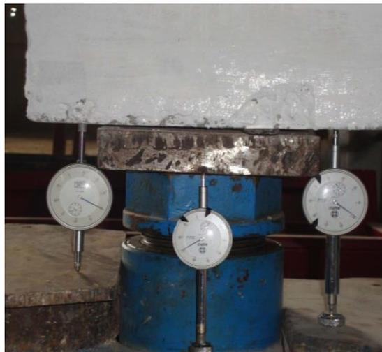
Plate (3): The testing measurements of Axial deformation.
