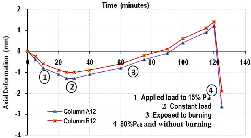
Figure (9): Axial deformation versus time curve at 50mm from the outer edge of column specimens A12 and B12 before, during and after burning at 400 °C.
