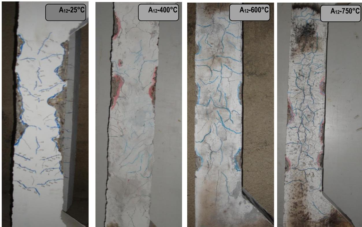
Plate (4): Typical crack pattern of series A column specimens before and after burning and subjected to concentric loading.
