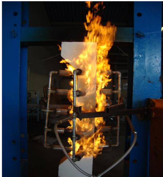
Plate (2): Testing of column specimens under 15% of ultimate load with exposure to fire flame.
