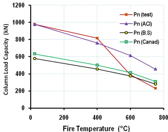
Figure (7): Effect of fire temperature on the axial load capacity of column specimens B<sub>12</sub>.
