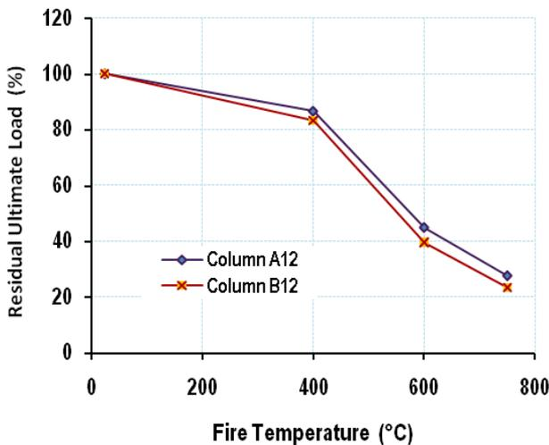
Figure (5): Effect of fire temperature on the residual axial load capacity of column specimens for series A and B.
