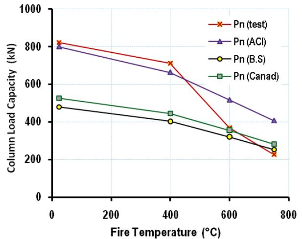
Figure (6): Effect of fire temperature on the axial load capacity of column specimens A<sub>12</sub>.
