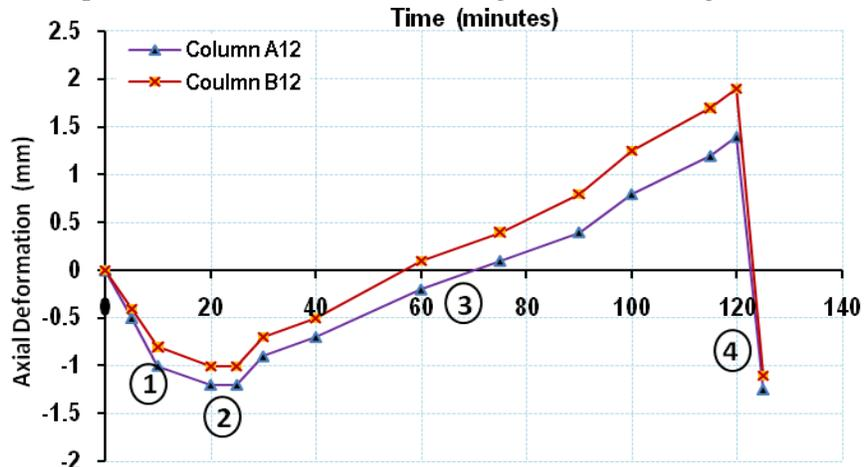
Figure (11): Axial deformation versus time curve at 50mm from the outer edge of column specimens A12 and B12 before, during and after burning at 750 °C.
