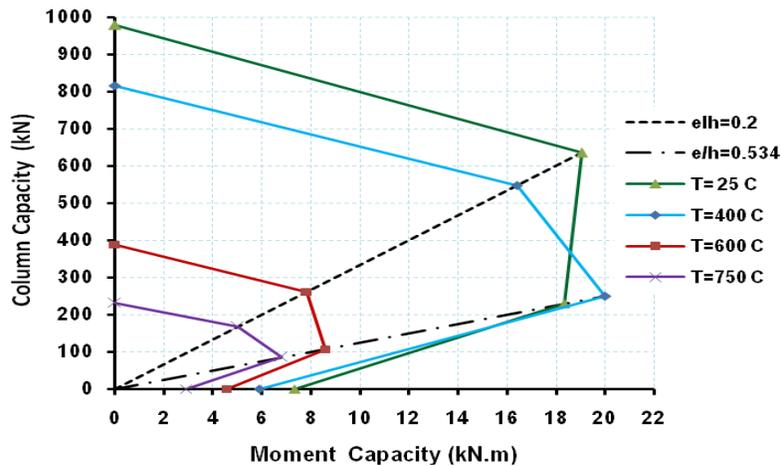
Figure (4): Effect of fire temperature on the interaction diagram of column specimens for series B and duration of burning 1.5 hour.
