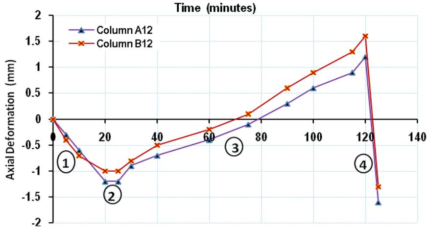
Figure (10): Axial deformation versus time curve at 50mm from the outer edge of column specimens A12 and B12 before, during and after burning at 600 °C.
