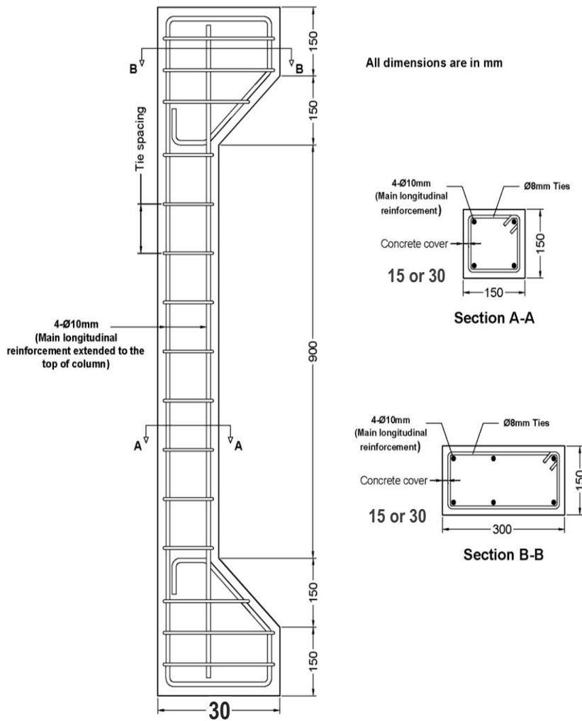
Figure (2): Reinforcement details of reinforced concrete column specimens.
