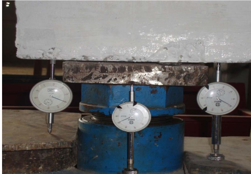
Plate (2): The testing measurements of Axial deformation.
