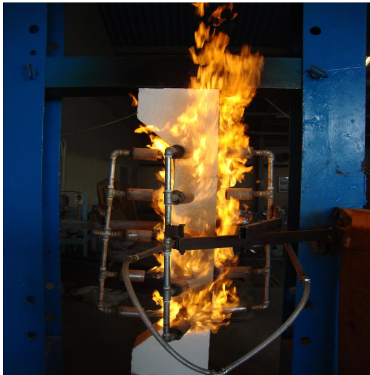
Plate (3): Testing of column specimens under 15% of ultimate load with exposure to fire flame.
