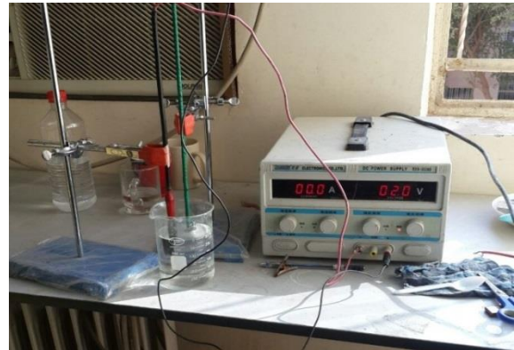
Figure1: Photograph of the complete assembly of the anodizing apparatus.
