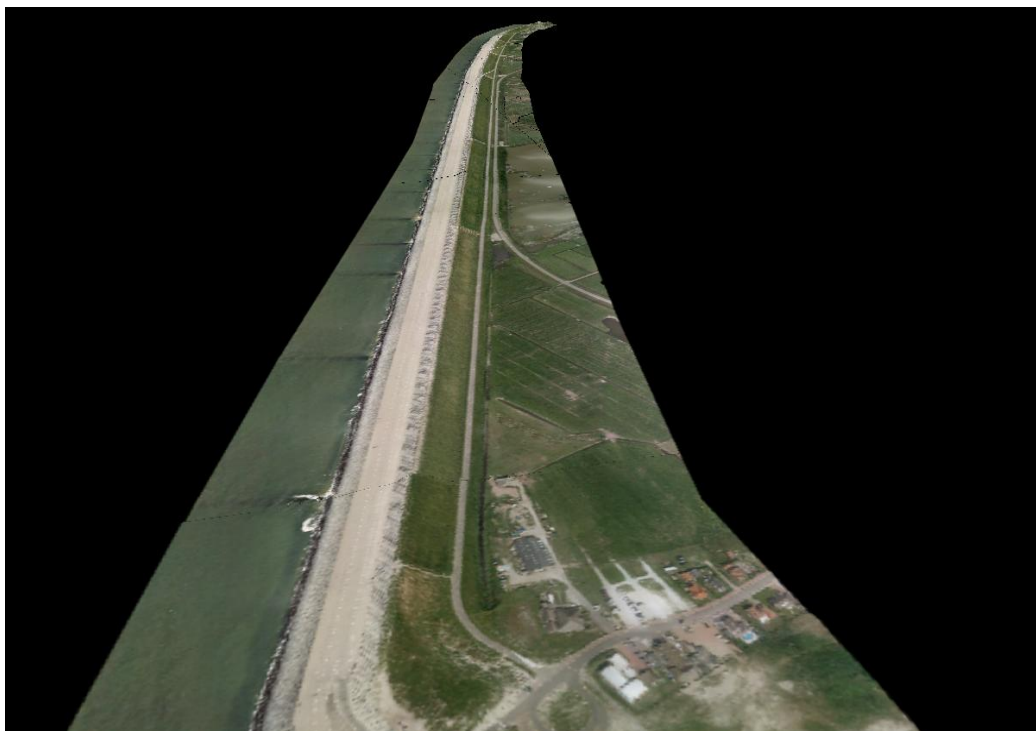
Figure (12) A side perspective view of the textured DTM showing the Hondsbosschezeewering dike
