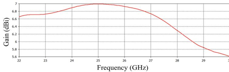
Figure 6: Gain Variation Over Frequencies Of the Suggested Single Element Patch Antenna.
