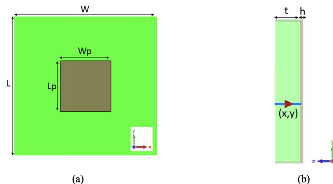
Figure 1: Geometry Of the Suggested Single Element Patch Antenna (a) Front View, and (b) Side View
