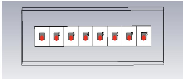
Figure 2: ULA Antenna Array Geometry
