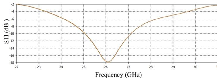
Figure 7:  $S_{11}$  Curve Of the Suggested 8 Element ULA Antenna Array.
