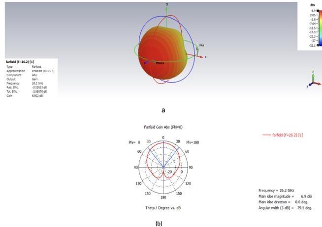
Figure 5: Far Field Radiation Pattern Of the Suggested Single Element Patch Antenna at 26.2GHz (a)2D and (b) 3D.
