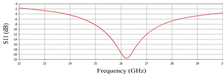
Figure 4: Curve Of the Suggested Single Element Patch Antenna.
