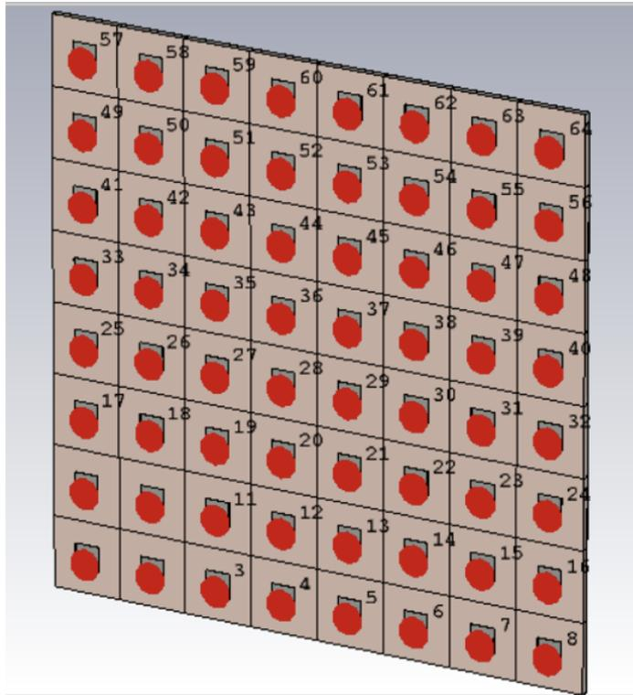
Figure 3: UPA Antenna Array Geometry
