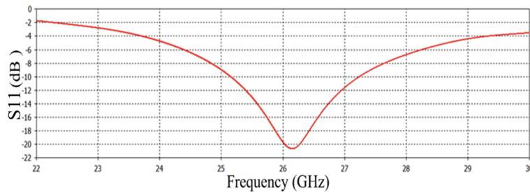
Figure 10:  $S_{11}$  Curve Of the Suggested  $8 \times 8$  Element UPA Antenna Array
