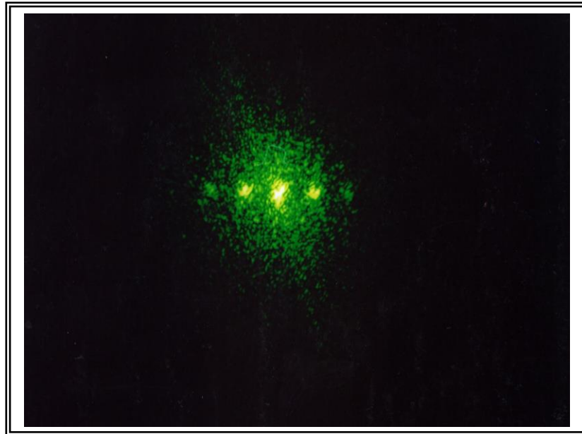
Fig (8): illustrates the orders of resultant diffraction by using the off-axis method at interfered angle 40^\circ .
