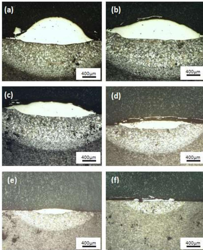
**Figure 2: Transverse cross sections of clad coatings showing the variation of the geometry dimensions at different specific energies (J/mm<sup>2</sup>) (a) 480, (b) 220, (c) 150, (d) 109, (e) 79 and (f) 58.**
