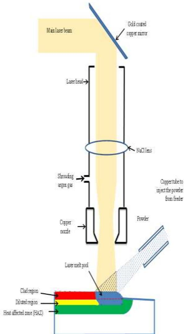
**Figure 1: Schematic diagram of laser head and principle of laser cladding showing the different features of clad coating.**
