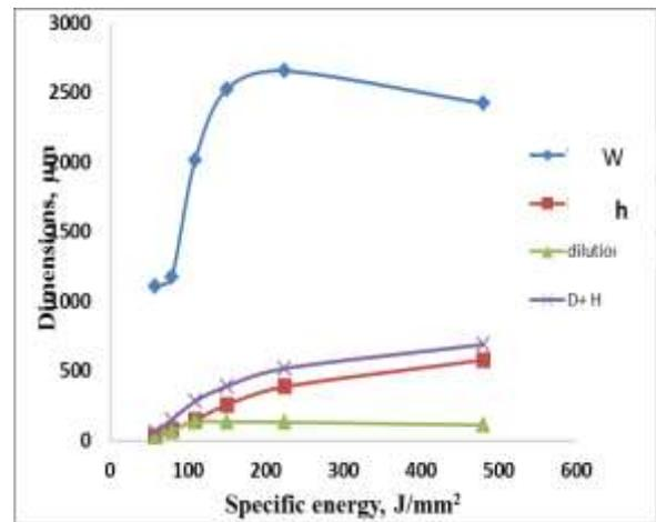
**Figure 6: Geometry dimensions of clad width (W), clad height (h), depth of dilution (d<sub>h</sub>) and total clad thickness (h + d<sub>h</sub>) as a function of specific energy for Ni-5 wt% powder clad on steel substrate.**
