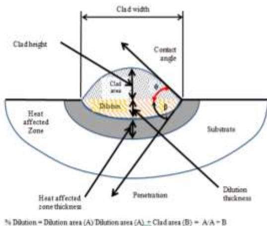
**Figure 5: Cross section view of the clad region showing the geometry dimensions and contact angle.**
