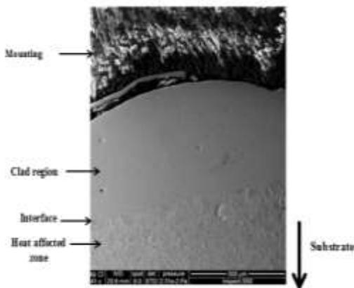
**Figure 4: SEM micrograph of transverse section of clad coating showing the sound clad region and sharp interface between clad and HAZ.**
