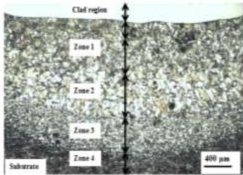
**Figure 3: General appearance of clad coating showing the different zones of heat affected zone.**
