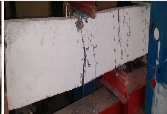
**Figure (27):** Specimen (1DB4) after testing.
