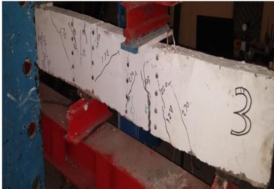
**Figure (26):** Specimen (1DB3) after testing.
