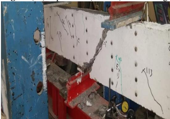
Figure (36): Specimen (1DB5S) after testing.
