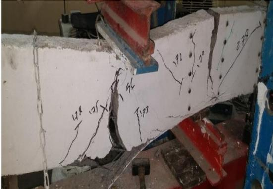
Figure (34): Specimen (1DB3S) after testing.
