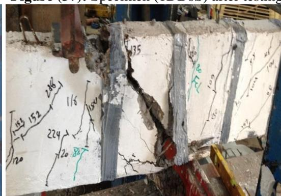
Figure (39): Specimen (1DB8S) after testing.
