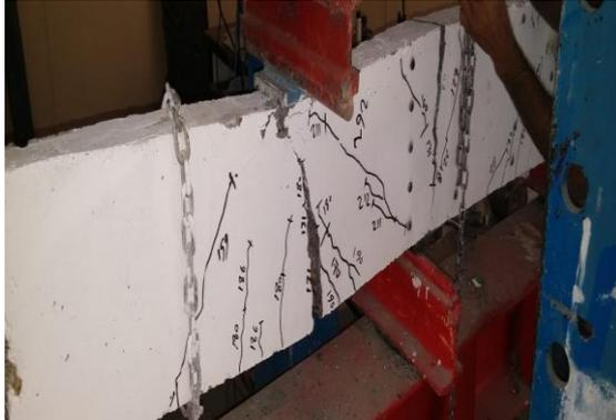
**Figure (28):** Specimen (1DB5) after testing.
