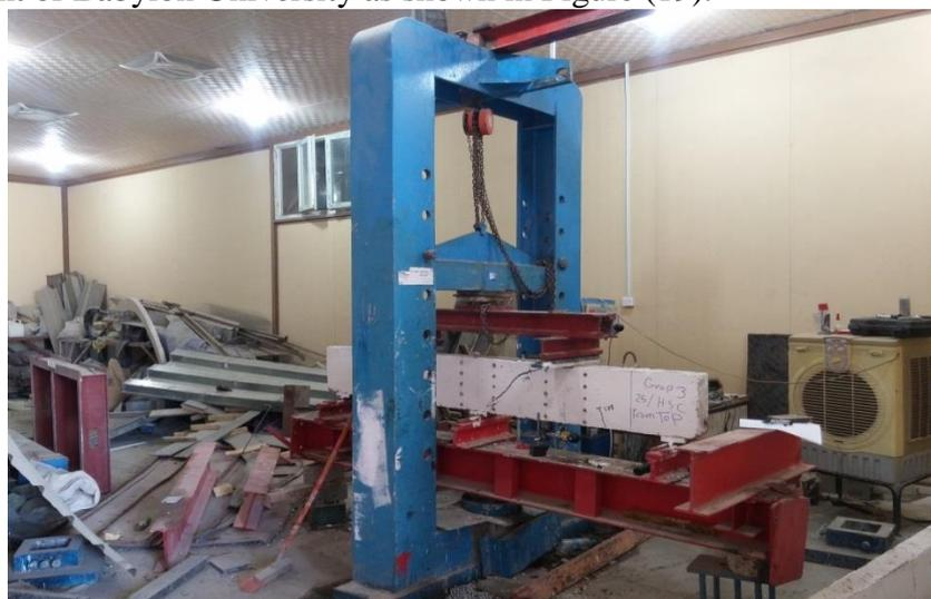
**Figure (19):** Hydraulic testing machine.
