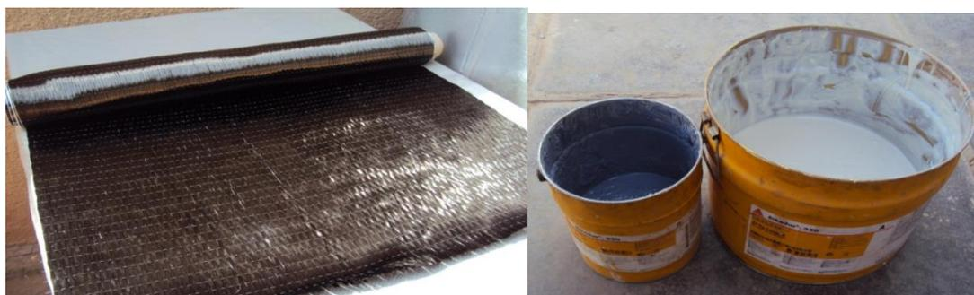
**Figure (18):** CFRP and epoxy used in strengthening of specimens.
