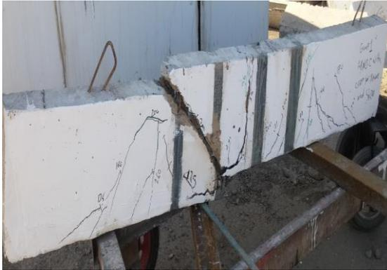
Figure (32): Specimen (1DB1S) after testing.
