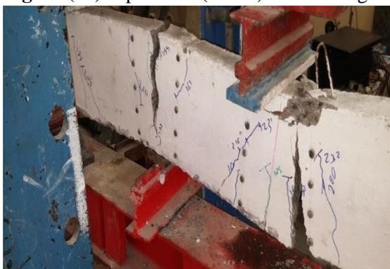
**Figure (30):** Specimen (1DB7) after testing.
