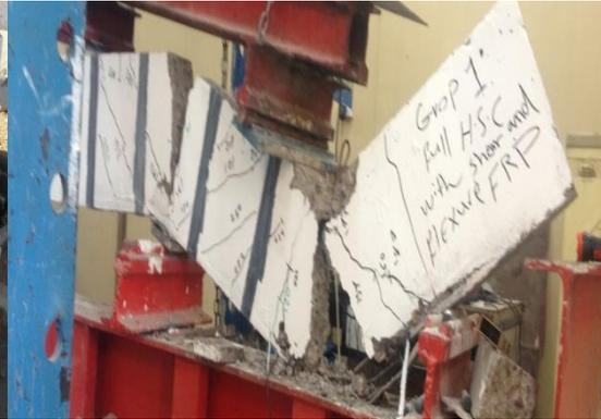
Figure (33): Specimen (1DB2S) after testing.
