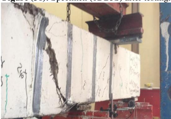
Figure (38): Specimen (1DB7S) after testing.
