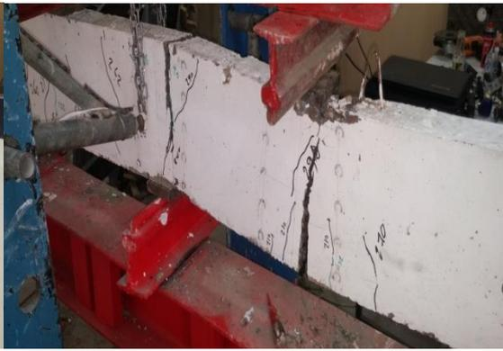
**Figure (25):** Specimen (1DB2) after testing.
