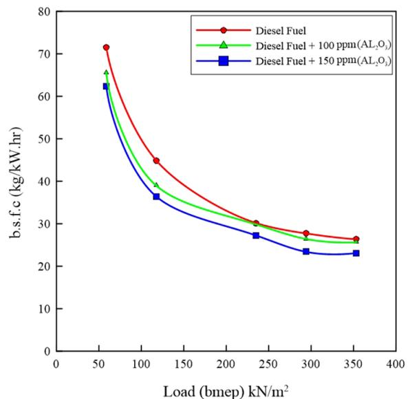
Figure 2: The brake specific fuel consumption (BSFC) at different loads for three types of fuels
