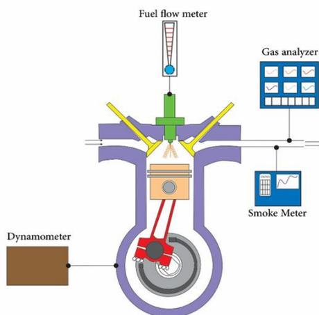
Figure 1: Schematic of the rig
