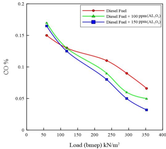
**Figure 6: The CO at different loads for three types of fuels**
