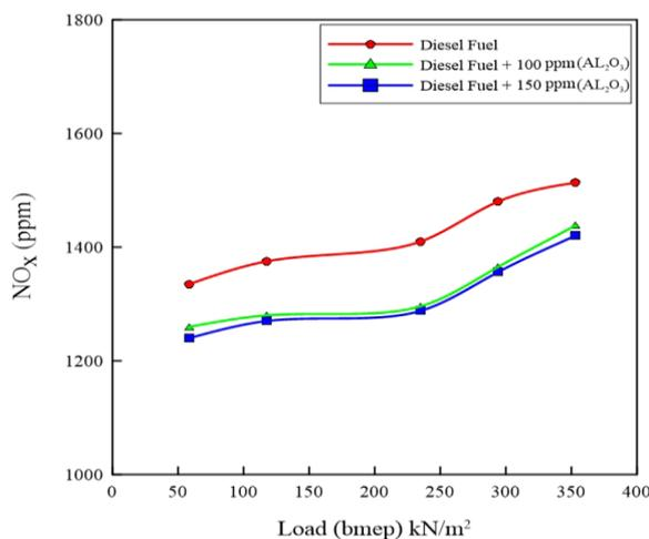
Figure 4: The NO<sub>x</sub> at different loads for three types of fuels.
