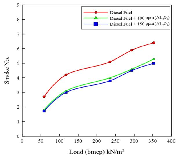
Figure 5: The Smoke NO at different loads for three types of fuels.
