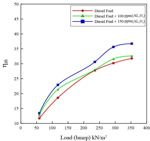
Figure 3: The brake thermal efficiency at different loads for three types of fuels.
