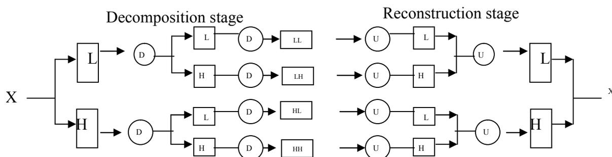
Figure 1: Image Wavelet decomposition tree using column and row two-dimensional signal decomposition with down sampling in each stage followed by image reconstruction, (for more details see [Prochazka et al,Witwit2001]).
