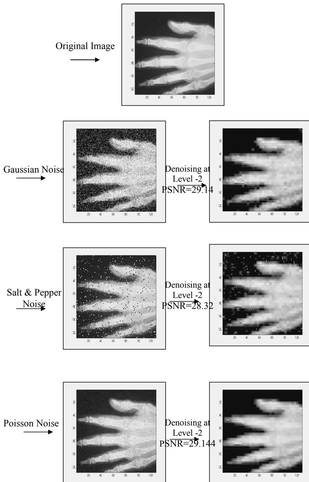
Figure (4) : illustrate results of denoising X-ray image(at Level-2) degraded by different noise using The modified Daubecheis Wavelet Transform .
