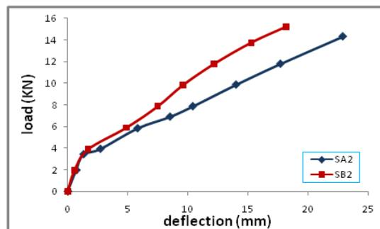
**Fig 5.1(b) Load- midspan deflection for Specimens (SA2:SB2)**
