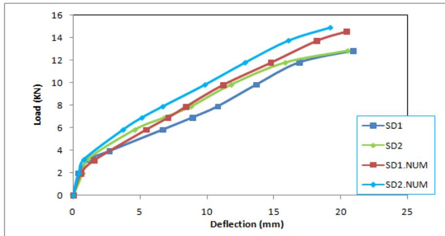
Fig 11.3 Load mid-span deflection for specimens (SD1:SD2)
