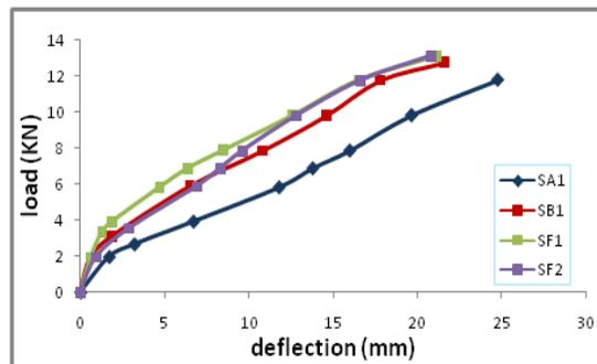
Fig.5.4 Load mid-span deflection for specimens (SA1:SB1:SF1:SF2)
