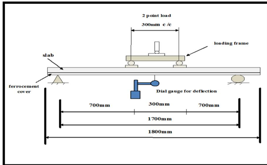
**Fig. 3: position of transducer, loading point**
