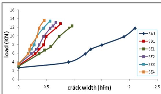
**Figure (7.1) Crack Width Versus Applied Load for Effect of Ferrocement Thickness**
