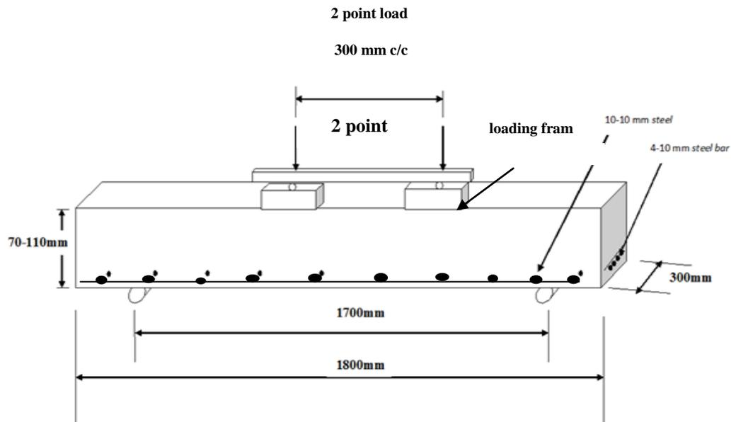
**Figure (1-1): Geometry of Laboratory Specimens**
