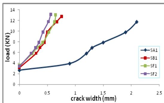
**Figure (7.3) Crack Width Versus Applied Load for Effect of Compressive Strength of Ferrocement**
