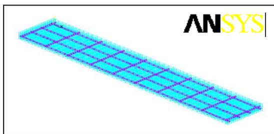
**Fig 9.3.: Internal reinforcement arrangement of tested concrete slabs**
