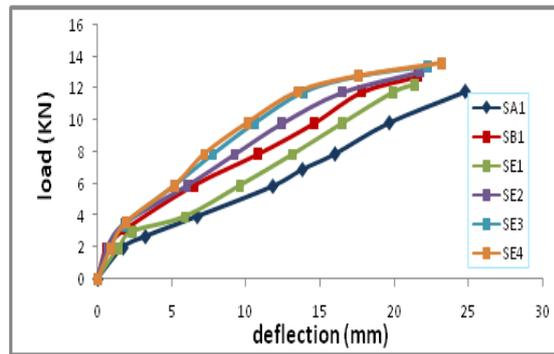
Fig.5.3 Load- midspan deflection for specimens (SA1:SB1:SE1:SE2:SE3:SE4)
