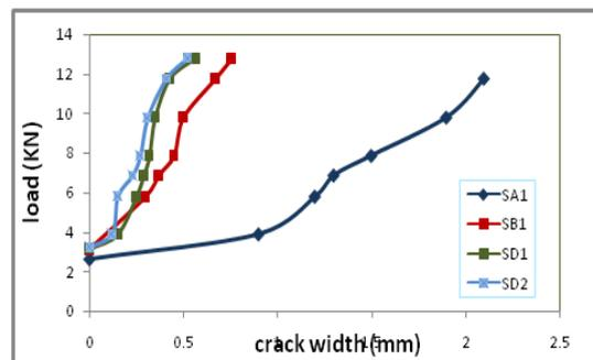
**Figure (7.2) Crack Width Versus Applied Load for Effect of Number of Wire Mesh**
