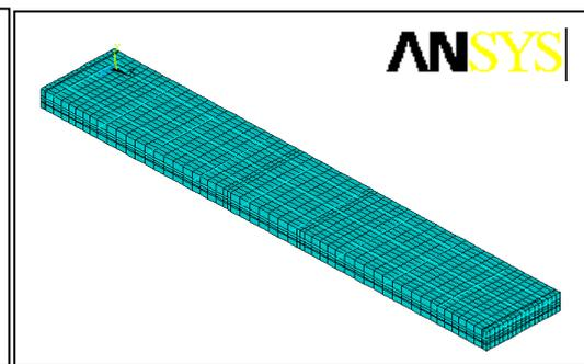
**Fig 9.2. : Mesh modeling of tested concrete slab (SB1)**
