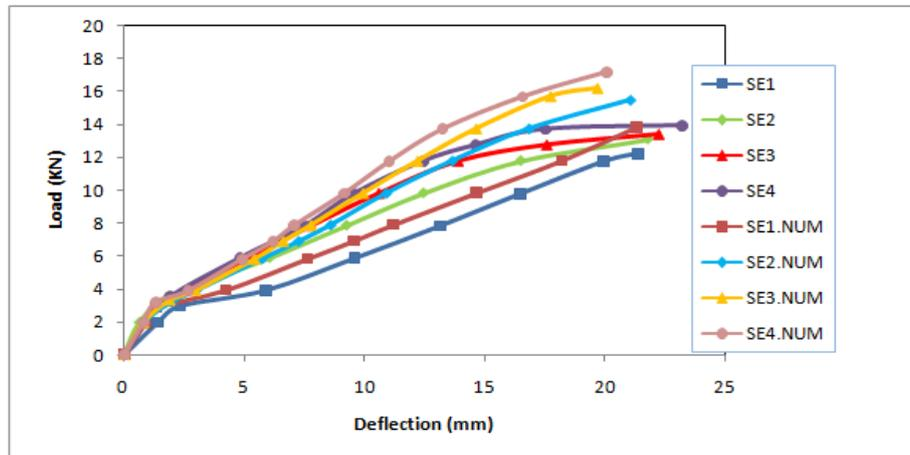
Fig 11.4. Load mid-span deflection for specimens (SE1:SE2:SE3:SE4)
