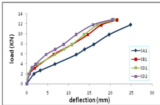
Fig.5.2 Load- midspan deflection for specimens (SA1:SB1:SD1:SD2)
