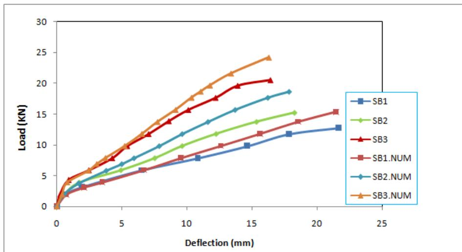
Fig 11.2. Load mid-span deflection for specimens (SB1:SB2:SB3)
