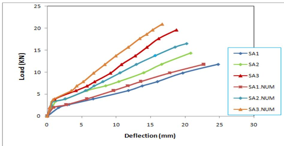
Fig 11.1. Load mid-span deflection for specimens (SA1:SA2:SA3)
