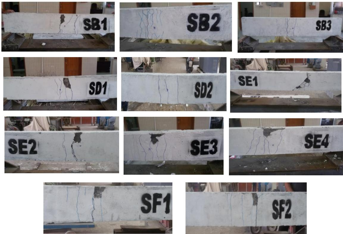
**Figure 8: Cracks Pattern of Slabs**
