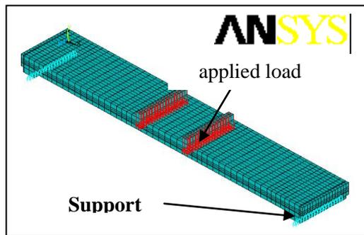
**Fig 9.1. Applied loads and Supports**
