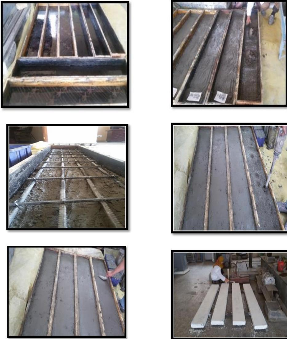
**Fig 2: Placing the wire mesh and casting the slabs**
