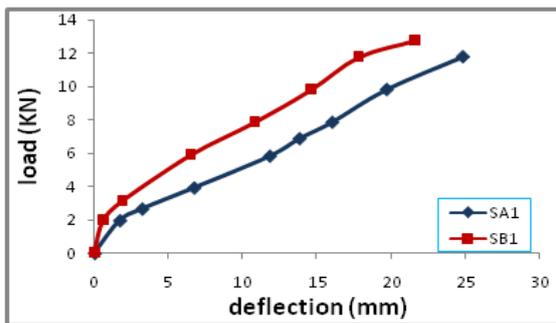
**Fig 5.1(a) Load- midspan deflection for specimens (SA1:SB1)**
