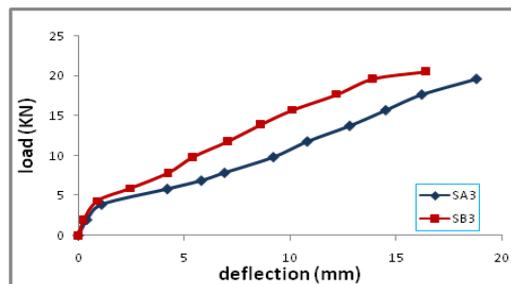
**Fig.5.1.(c) Load- midspan deflection for specimens (SA3:SB3)**
