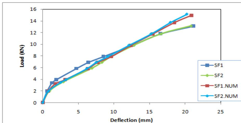
Fig 11.5 Load mid-span deflection for specimens (SF1:SF2)
