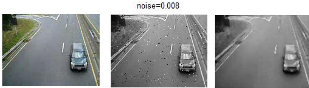
a) Original Image b) Image with Noise c) Output Image of Median Filter
