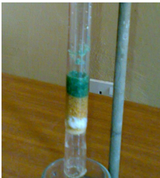
Figure 8: Picture show the efficiency of removal of MB on Can Papyrus for 0.6g (2.4cm), 15ppm and 12.5ml/min
