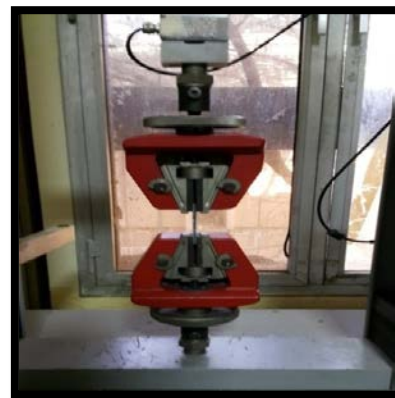
Figure (3): The tensile test machine (Testometric)
