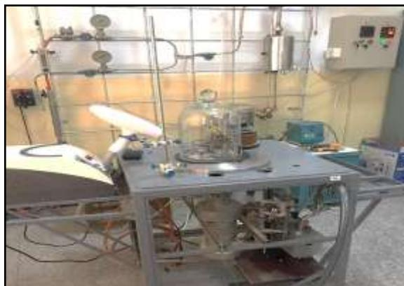
**Figure 2: The thin film preparation unit using PLD technique.**
