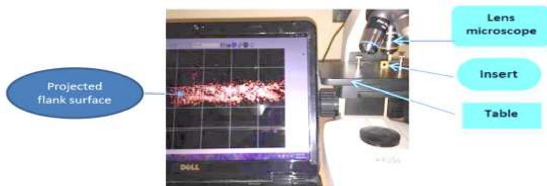
**Figure 1: Measurement flank wear to (SNMG0903) insert**
