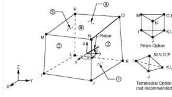
Figure (1) Solid (65) element [(9) ANSYS Manual]
