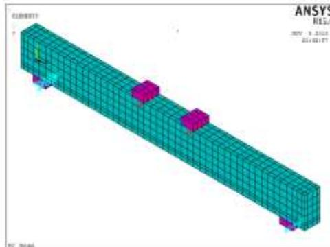
Figure (9) The boundary conditions of the specimens
