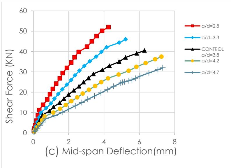
Figure (15) Effect of shear span-depth ratio on a) SP1 b) SP2 c) SP3.
