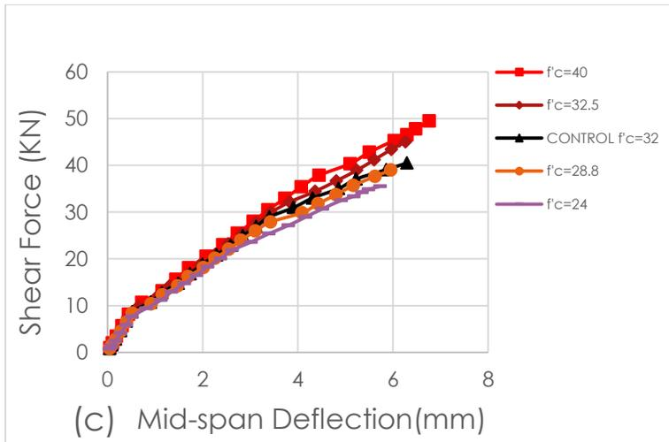
Figure (14) Effect of concrete compressive strength on a) SP1 b) SP2 c) SP3.
