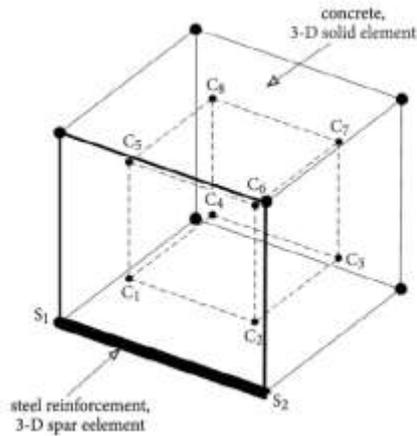
Figure (8) Discrete model for steel reinforcement.
