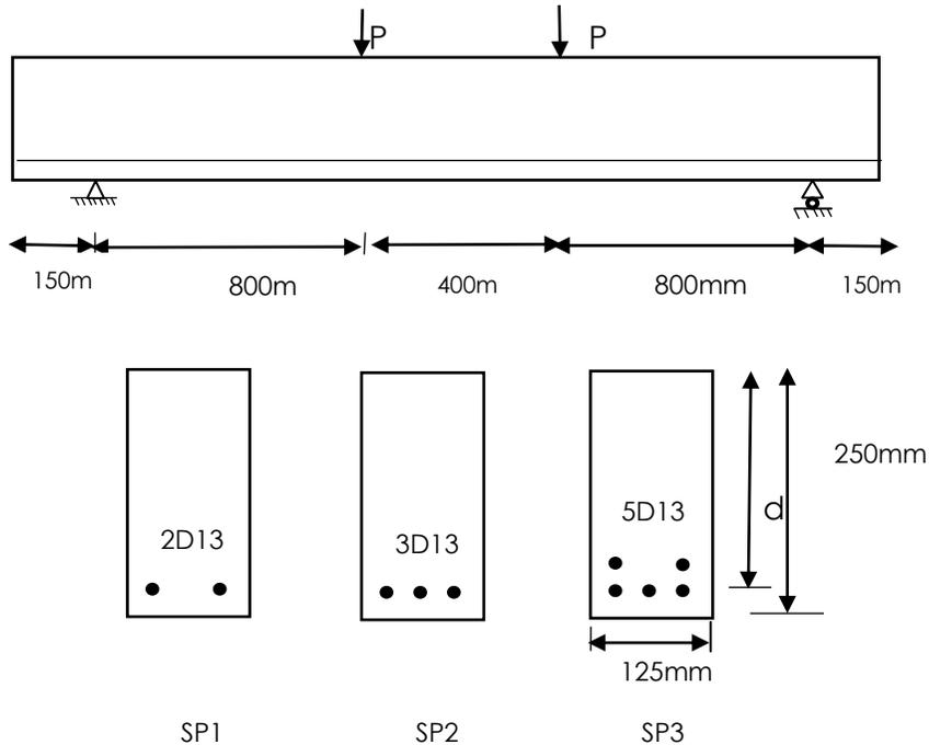
Figure (6) Dimensions of the specimens
