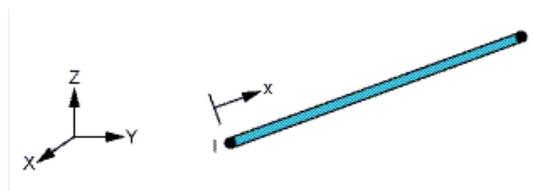
Figure (2) Link (180) element [(9) ANSYS Manual]
