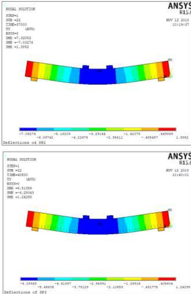
Figure (11) The variation of vertical displacement along the beams (SP1, SP2 and SP3) at ultimate shear force.
