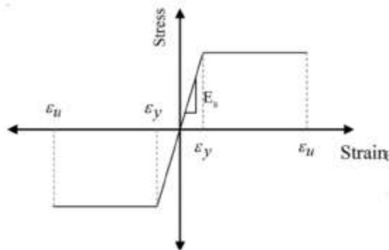
Figure (5) Uniaxial stress-strain curve for steel reinforcement
