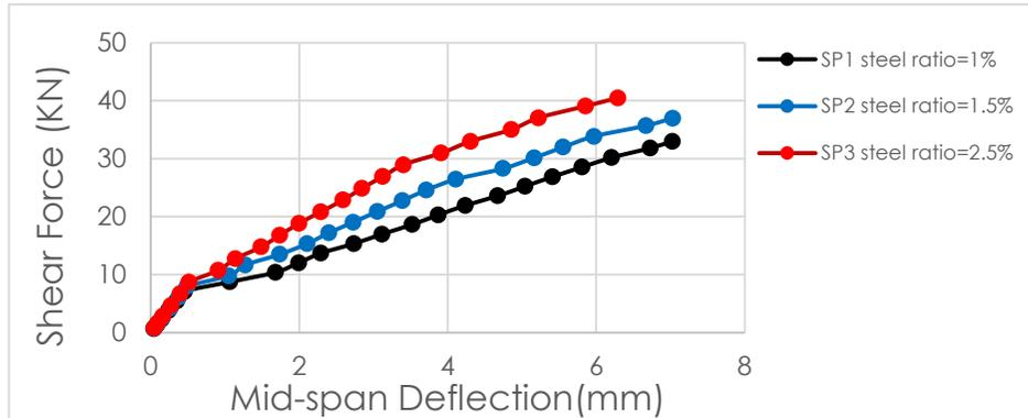
Figure (12) Effect of steel ratio ( $\rho\%$ ) on RC beams
