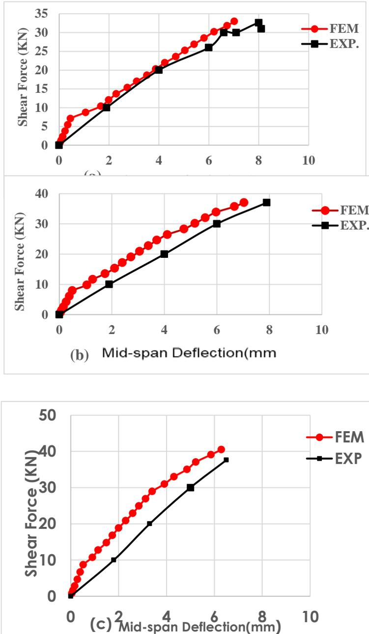
Figure (10) Shear force-mid-span deflection for a) SP1, b) SP2 and c) SP3
