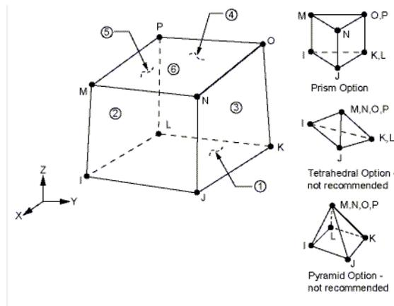
Figure (3) Solid (185) element [(9) ANSYS Manual]
