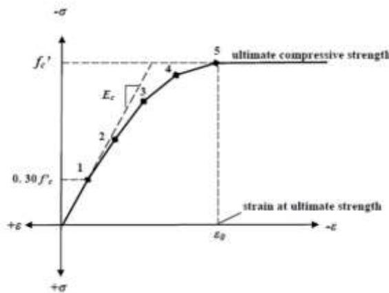
Figure (4) Typical uniaxial stress-strain curve for concrete in compression
