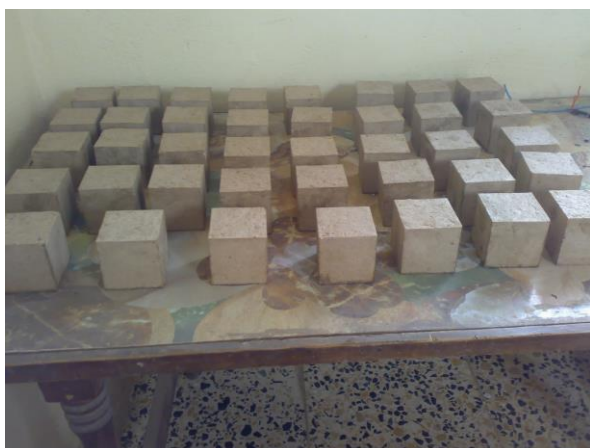
Picture (1): Ordinary gypsum specimens before heating.
