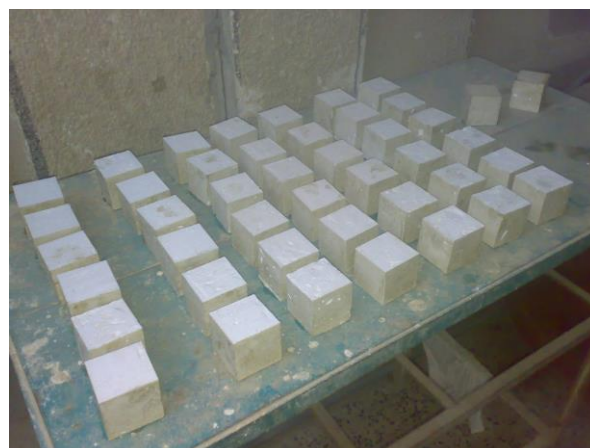
Picture (2): Plaster of Paris specimens before heating.
