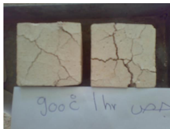
Picture (4): Cracks of ordinary gypsum specimens at failure.
