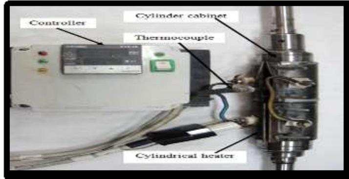
Figure (1) Heating system for tensile test specimen
