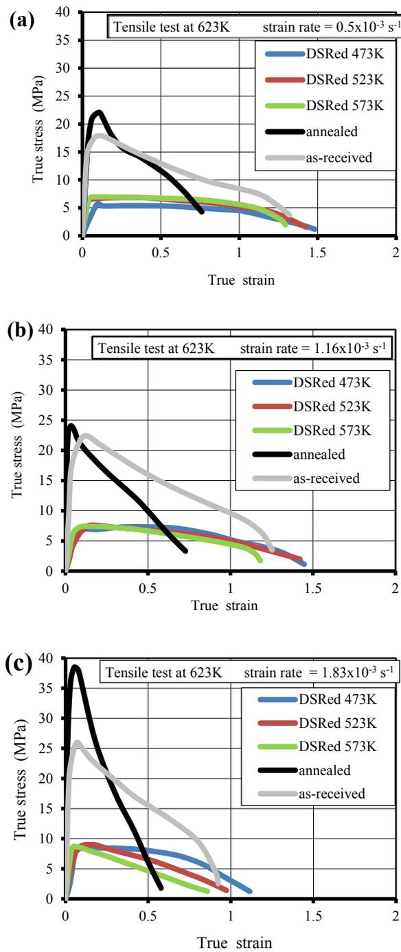
Figure (8) True stress- strain curves of AZ31B specimen at different initial strain rate (a)  $0.5 \times 10^{-3} \text{ s}^{-1}$  (b)  $1.16 \times 10^{-3} \text{ s}^{-1}$  (c)  $1.83 \times 10^{-3} \text{ s}^{-1}$ .
