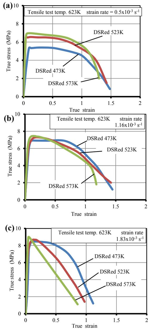
Figure (6) True stress- strain curves of tensile test for different DSRed specimens and constant initial strain rate (a)  $0.5 \times 10^{-3} \text{ s}^{-1}$  (b)  $1.16 \times 10^{-3} \text{ s}^{-1}$  (c)  $1.83 \times 10^{-3} \text{ s}^{-1}$
