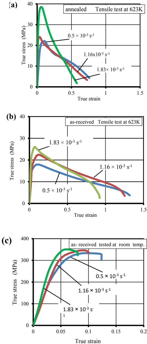
Figure (7) True stress- strain curves of tensile test at different initial strain rates and different AZ31B specimens (a) annealed test at 623K (b) as-received test at 623K (c) as-received at RT.
