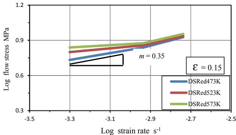
Figure (9). The  $\log \dot{\epsilon}$  vs.  $\log \sigma$  curves of the AZ31B alloy
