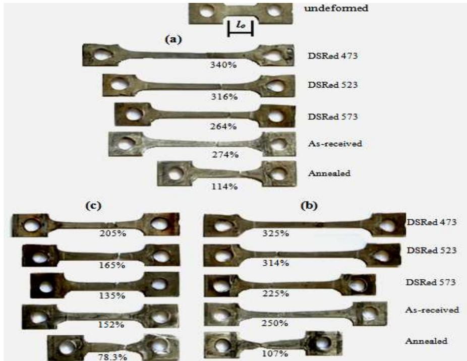
Figure (4) Tensile test at 623 K for various grain sizes of AZ31B specimens and constant initial strain rates (a)  $0.5 \times 10^{-3} \text{ s}^{-1}$  (b)  $1.16 \times 10^{-3} \text{ s}^{-1}$  (c)  $1.83 \times 10^{-3} \text{ s}^{-1}$ .
