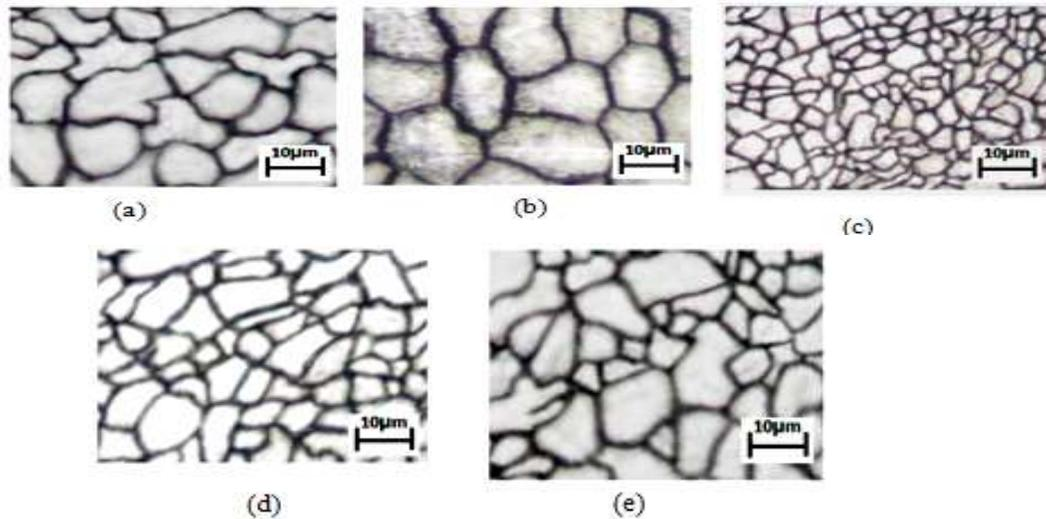
**Figure (2) Microstructure of the AZ31B magnesium alloy sheets specimens (a) as-received (b) annealed (c) DSRed 473K (d) DSRed 523K (e) DSRed 573K.**
