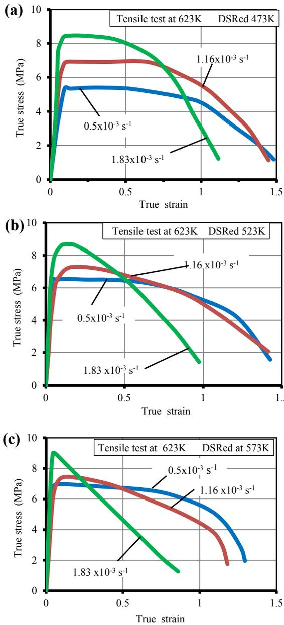
Figure (5) True stress- strain curves of tensile test at different initial strain rates for AZ31B specimens (a) DSRed 473K (b) DSRed 523K (c) DSRed 573K.
