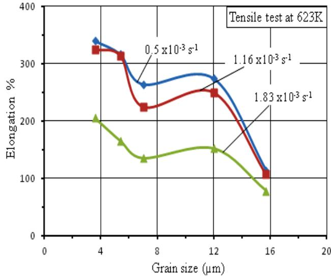
Figure (3) Elongation to failure as a function of grain size at temperature of 623K for AZ31B magnesium alloy specimens for different initial strain rate.
