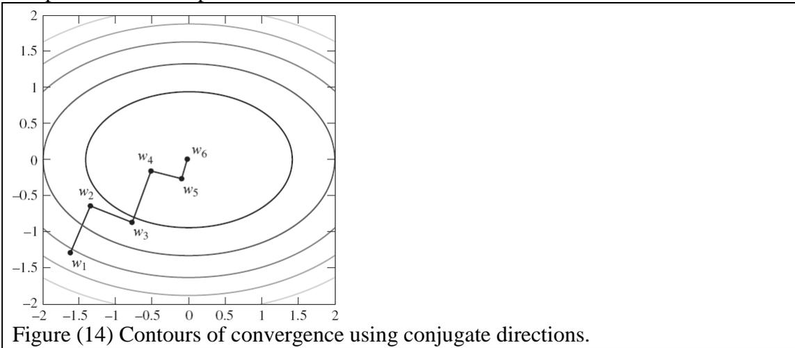
Figure (14) Contours of convergence using conjugate directions.
