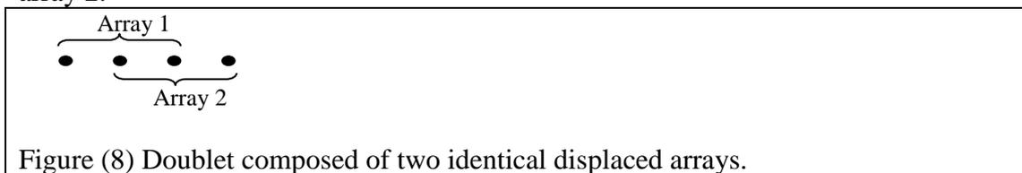
Figure (8) Doublet composed of two identical displaced arrays.
