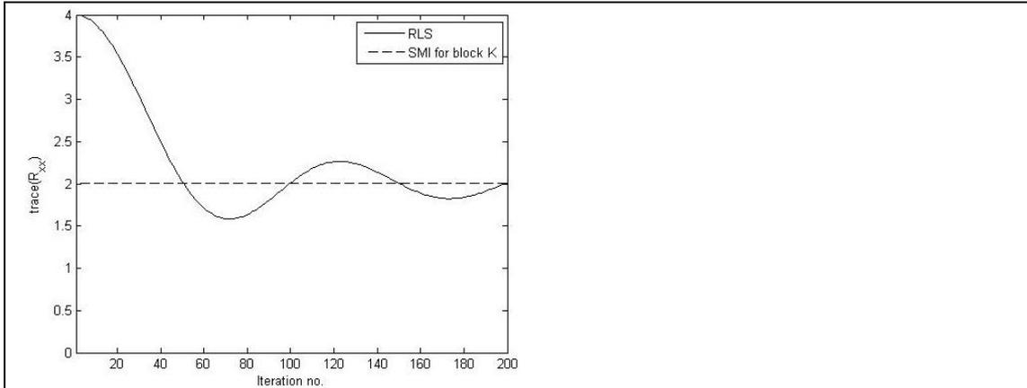
Figure (12) Trace of correlation matrix using SMI and RLS.
