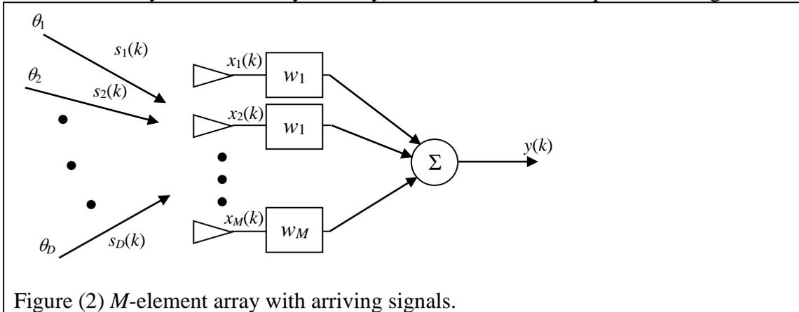
Figure (2)  $M$ -element array with arriving signals.
