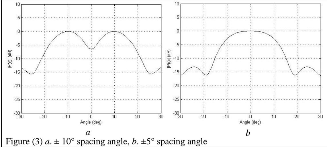
Figure (3) a.  $\pm 10^\circ$  spacing angle, b.  $\pm 5^\circ$  spacing angle
