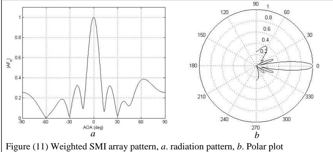
Figure (11) Weighted SMI array pattern, a. radiation pattern, b. Polar plot
