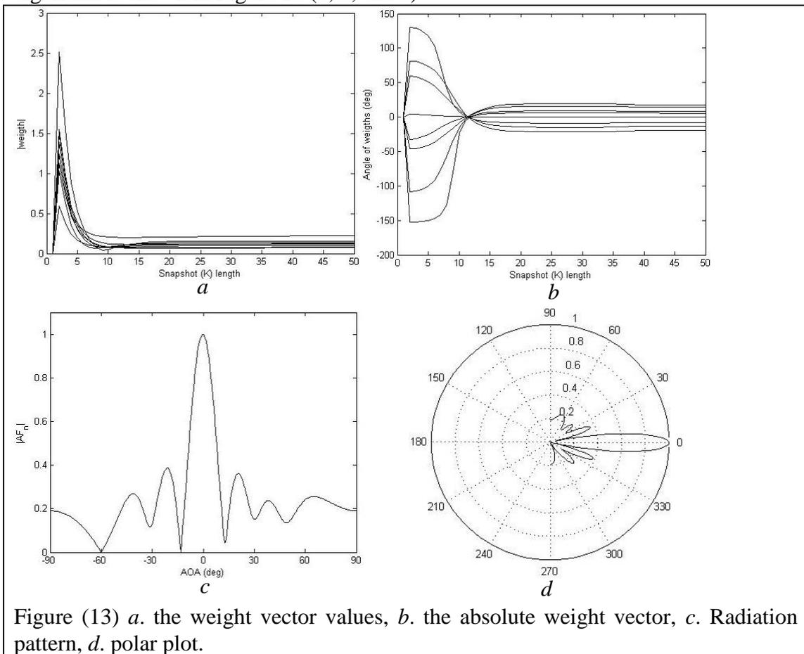
Figure (13) *a*. the weight vector values, *b*. the absolute weight vector, *c*. Radiation pattern, *d*. polar plot.
