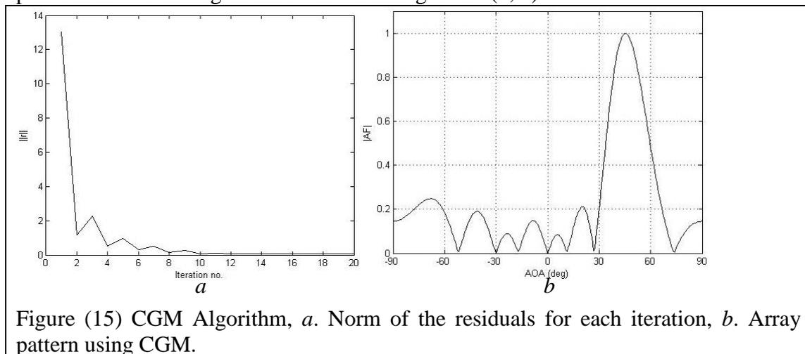
Figure (15) CGM Algorithm, a. Norm of the residuals for each iteration, b. Array pattern using CGM.
