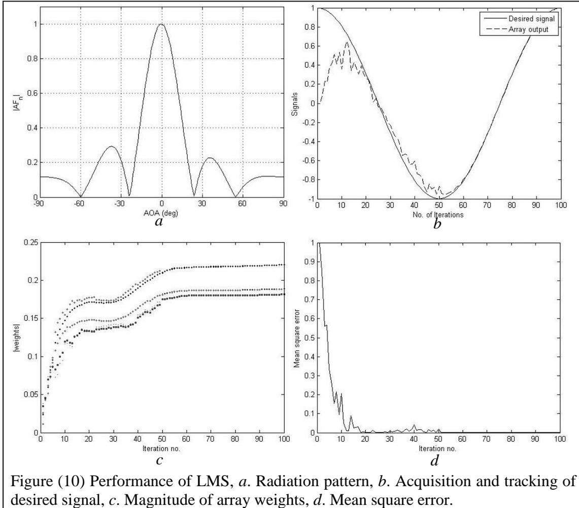
Figure (10) Performance of LMS, a. Radiation pattern, b. Acquisition and tracking of desired signal, c. Magnitude of array weights, d. Mean square error.
