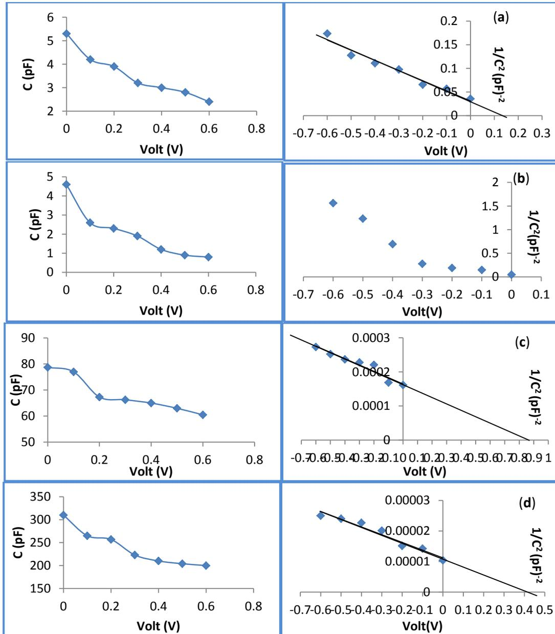
Figure(7): The variation of  $1/C^2$  versus reverse bias voltage for ZnS/Si heterojunction at different treatment temperatures (a) 50 C° (b) 100C° (c) 150C° (d) 200 C°
