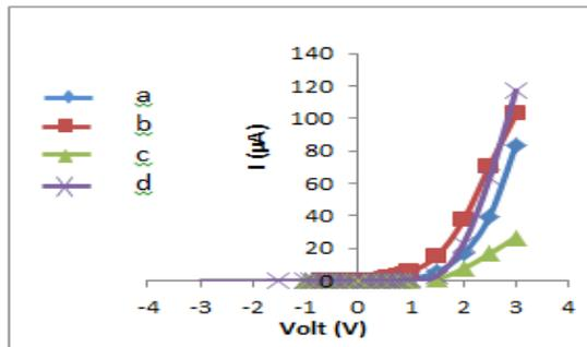
**Figure (5): I-V characteristics for ZnS heterojunction prepared at various substrate temperatures (a) 50, (b) 100, (c) 150 (d) 200C°**
