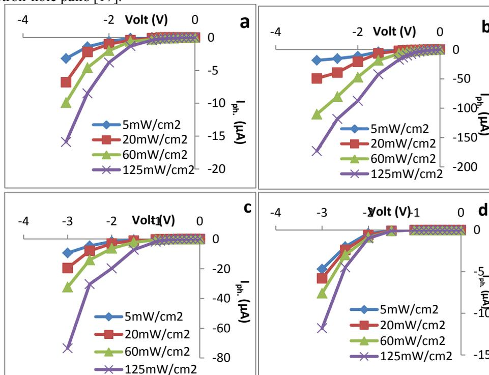
**Figure (6):  $I_{ph}$ - $V$  characteristics for ZnS/Si heterojunction at reverse bias voltage at various substrate temperatures (a) 50C° (b) 100C° (c) 150C° (d) 200 C°**
