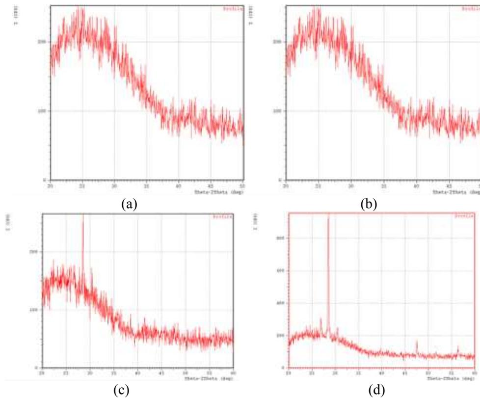
Figure ( 1 ) : XRD patterns of ZnS films grown at substrate temperatures (a) 50, ( b) 100 (c) 150 and (d) 200C°.
