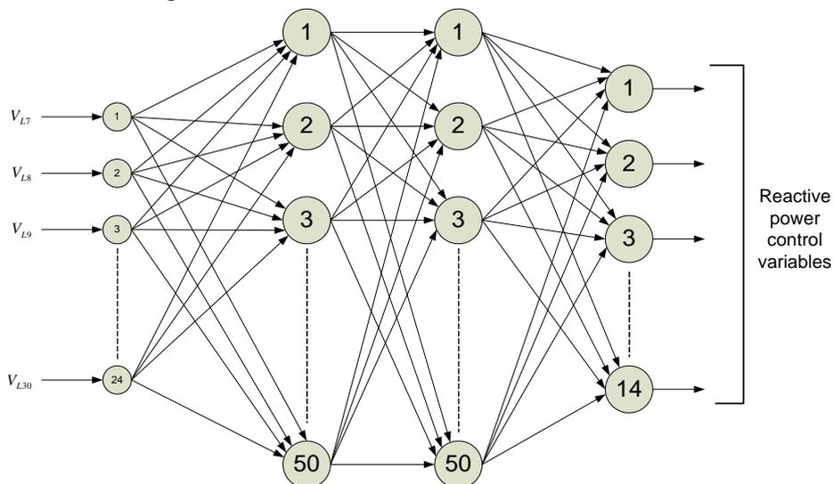
**Figure (2), Structure of neural network concerning IEEE 30-bus test system**
