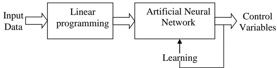
**Figure (1), The block diagram of the ANN-based algorithm for improving voltage stability in power systems**
