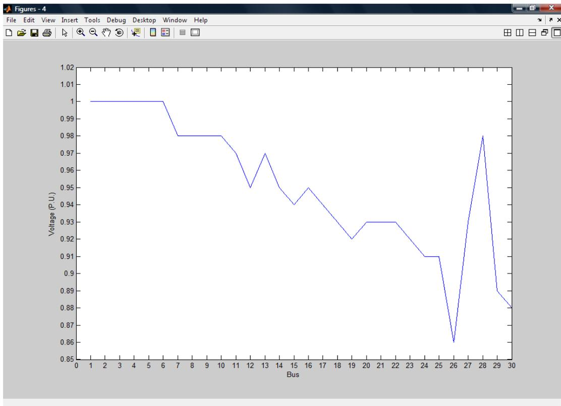
Figure (4), The pre optimization voltage profiles at each bus of the system under test.
