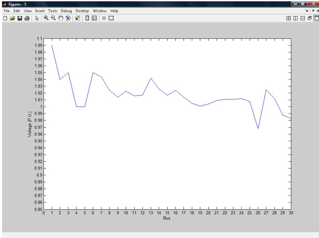
**Figure (5), The post optimization voltage profiles at each bus of the system under test.**
