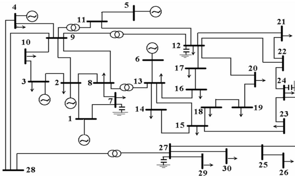
Figure (3), The modified IEEE 30-Bus Test System
