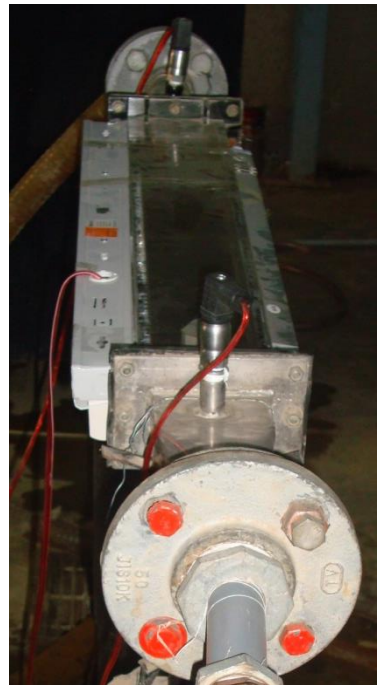
Fig (3) The test section(rectangular microchannel)
