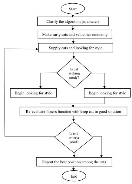
FIGURE 1. - Flow chart of cat optimization algorithm
