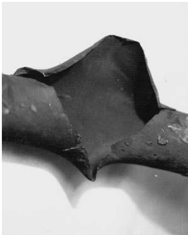
Fig. 5 The fracture exhibits {Cobra } appearance
