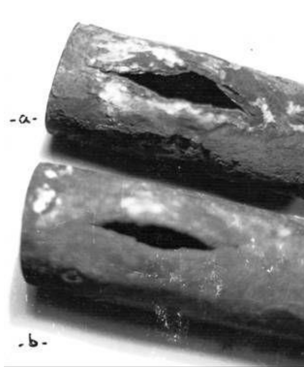
Fig.2. Over – all view of rupture. Atypical Fish Mouth rupture.
