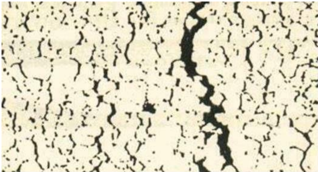
Fig.4 Intergranular nature of cracking for etched specimen electrolytically in 60% \text{HNO}_3 .
