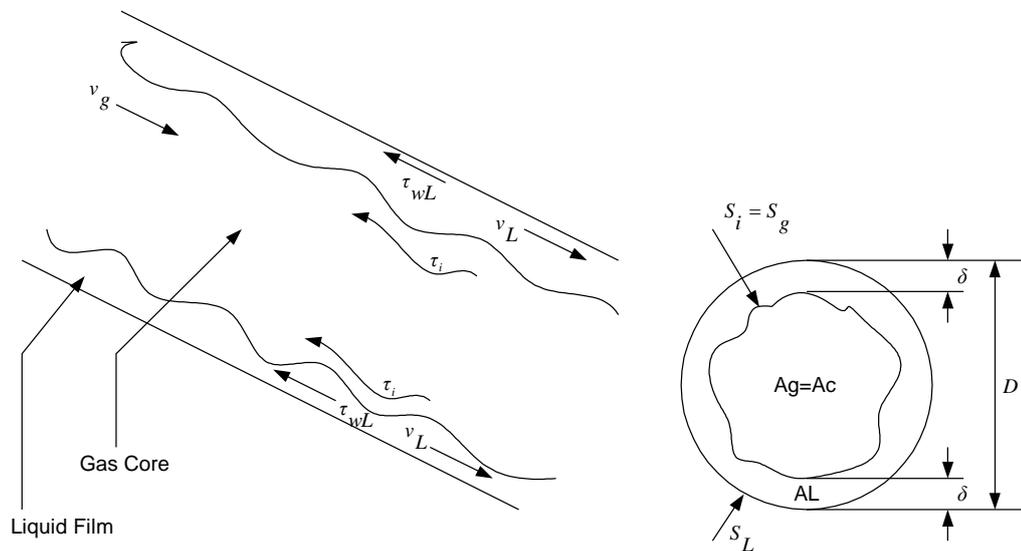
**Figure (1): Annular Flow Pattern Configuration**
