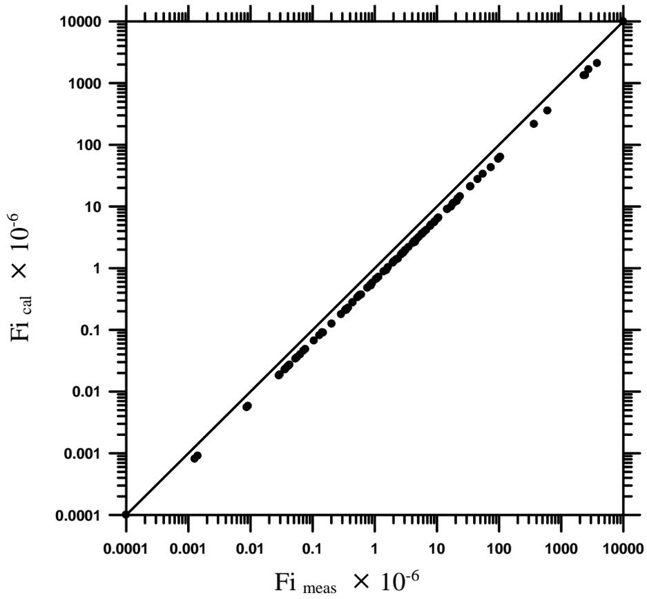
Figure (6): The distribution of the prediction interfacial friction factor by using the overall data (horizontal and inclined tests)
