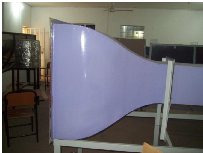
Fig. (6) Photograph settling chamber
