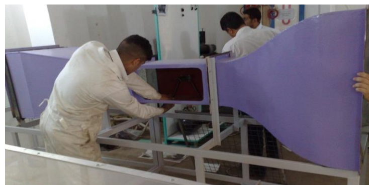
Fig. (10) Joining the wind tunnel
