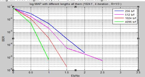
Fig. 6 : log-MAP technique with different code lengths
