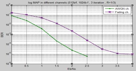
Fig.9 : log-MAP technique in different channels
