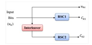
Fig. 1 : The structure of turbo encoder
