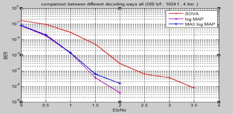
Fig.5 : Turbo code in three decoding techniques
