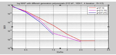
Fig. 8 : Turbo code with different generators polynomials in log-MAP technique
