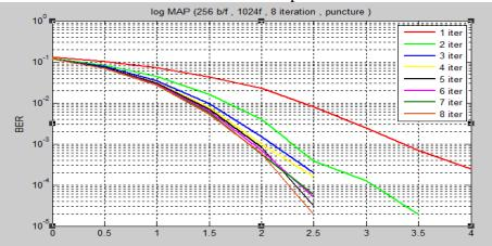
Fig. 4 : performance of turbo code with 8 iteration Table(2) illustrates the value of BER at  $Eb/No = 2 \ dB$  for each iteration. Table (2): BER at different number of iteration
