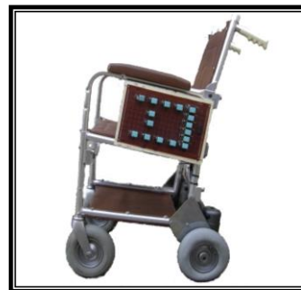
Figure (4), Relay Interfacing Fixated on Wheelchair
