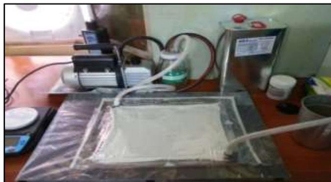
**Figure (3): Vacuum bagging technique.**
