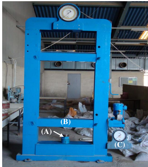
Plate (1): Flexural strength testing machine.
