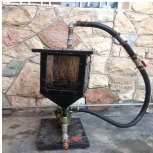
**Figure (1) Erosion device**
