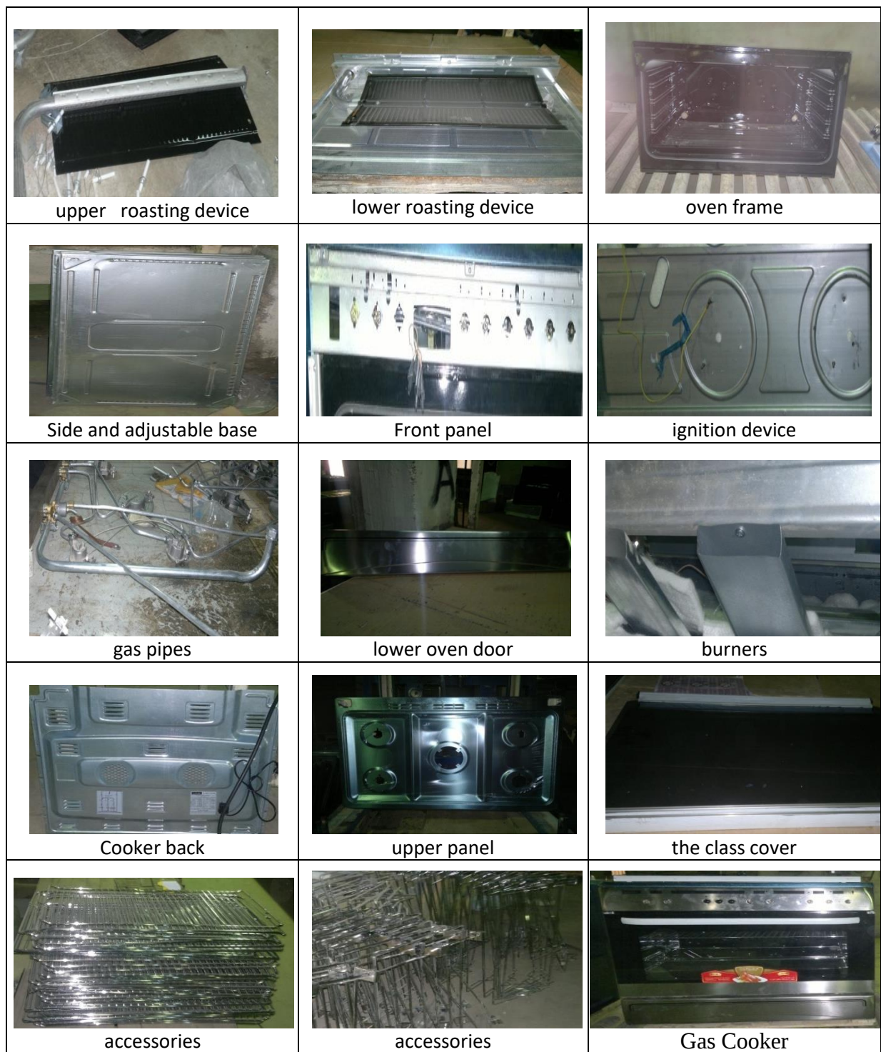
Figure(1) gas cooker parts.
