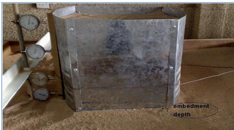
Fig. (10): Cellular retaining structure in case embedment depth
