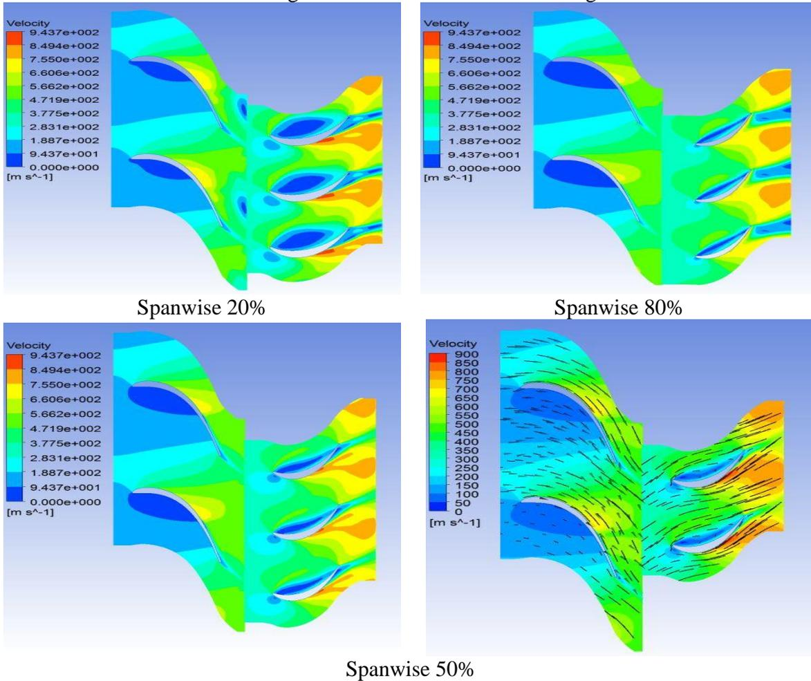
Figure 7: Velocity Contours & Stream Lines for Different Span
