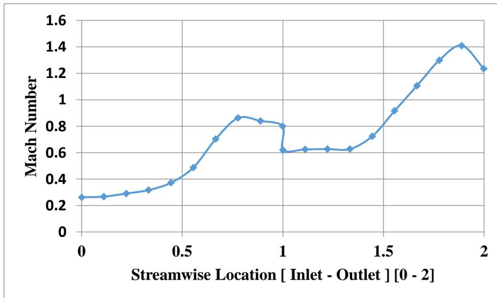
**Figure 9: Mach number with Streamwise Location from Inlet to Outlet**
