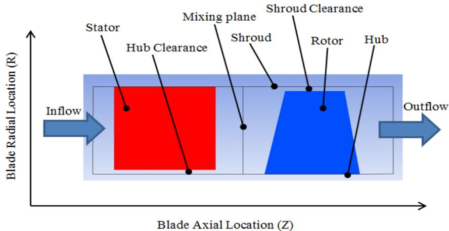
**Figure 1: Rotor and stator on the Meridional View(Ansys Blade Modular)**
