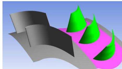
Rotor( blade and hub):which is the wall moving boundary
