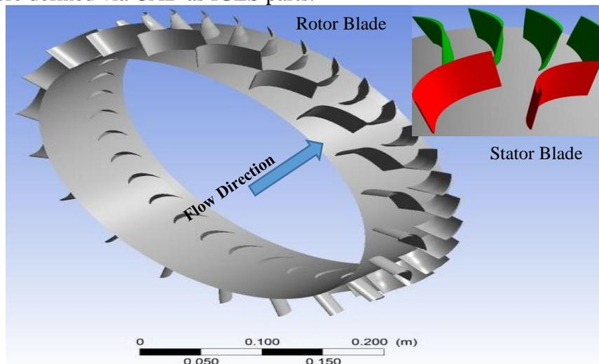
**Figure 2: Three Dimensional View of an Axial Turbine stage**
