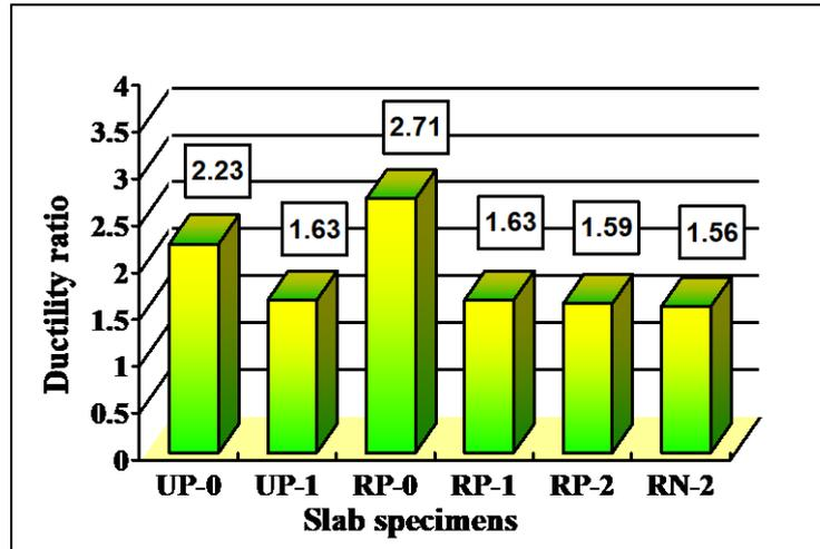
Figure (10): Ductility ratio for the tested slabs
