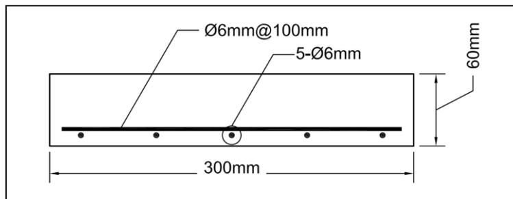
Figure (2): Cross-section of bare concrete slab
