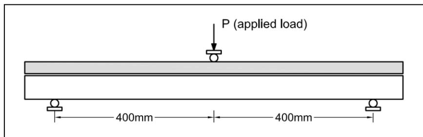
**Figure (6): Test setup for slab specimens**
