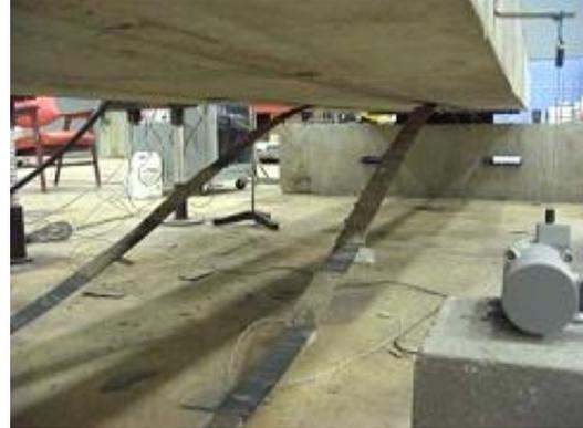
(b): CFRP debonding
