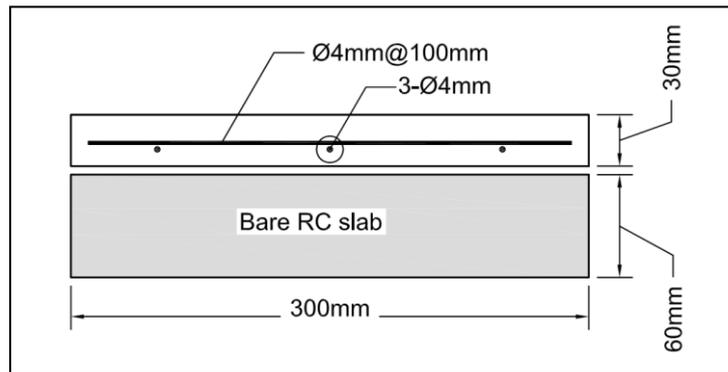
**Figure (3): Reinforcement details of the concrete overlay**
