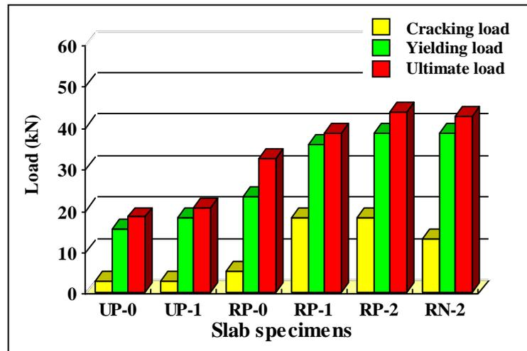
Figure (8): Comparison between slab specimens at different loading stages
