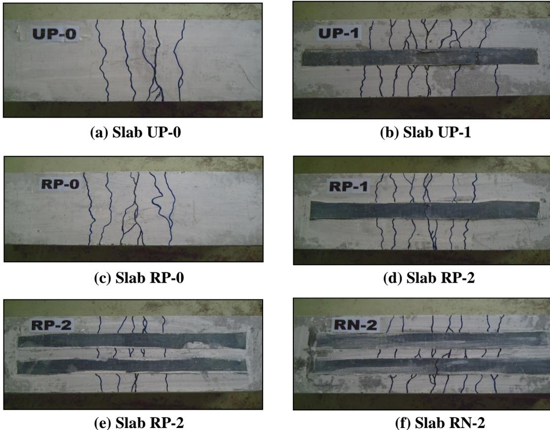
Figure (9): Crack patterns after failure for the slab specimens
