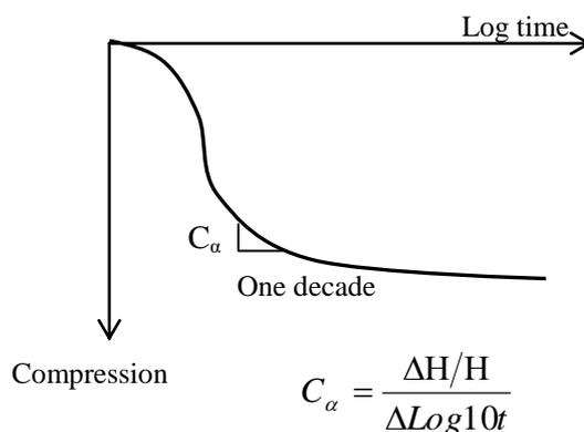
**Figure (1): Definition of Rate of Secondary Compression**
