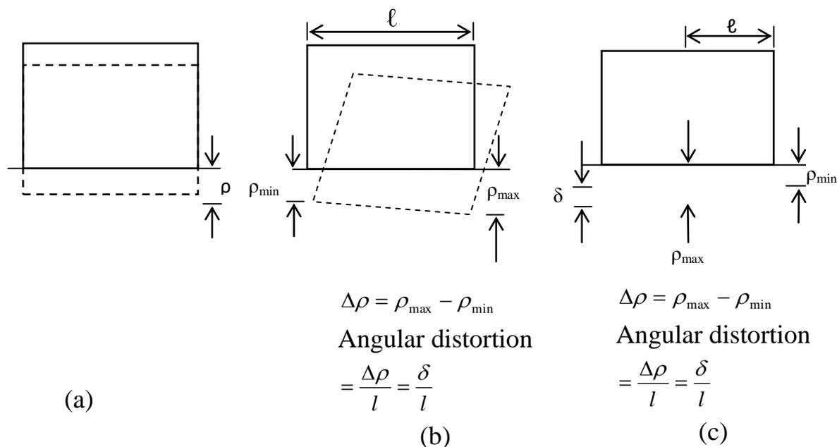
Figure (2) Types of Settlement (a) Uniform Settlement (b) Tilt (c) Non-Uniform Settlement (Lambe and Whitman 2008)
