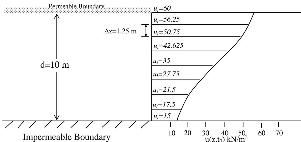
**Figure (5): Initial Excess Pore-Water Pressure**
