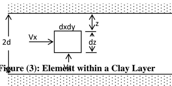
Figure (3): Element within a Clay Layer
