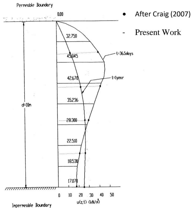
**Figure. (6) Excess Pore Water Pressure at The End of The 2<sup>nd</sup> and 20<sup>th</sup> Time Steps**
