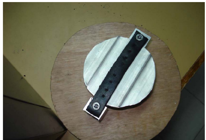
Figure (4): Cylindrical Piece With strip of plastic For Clamping.
