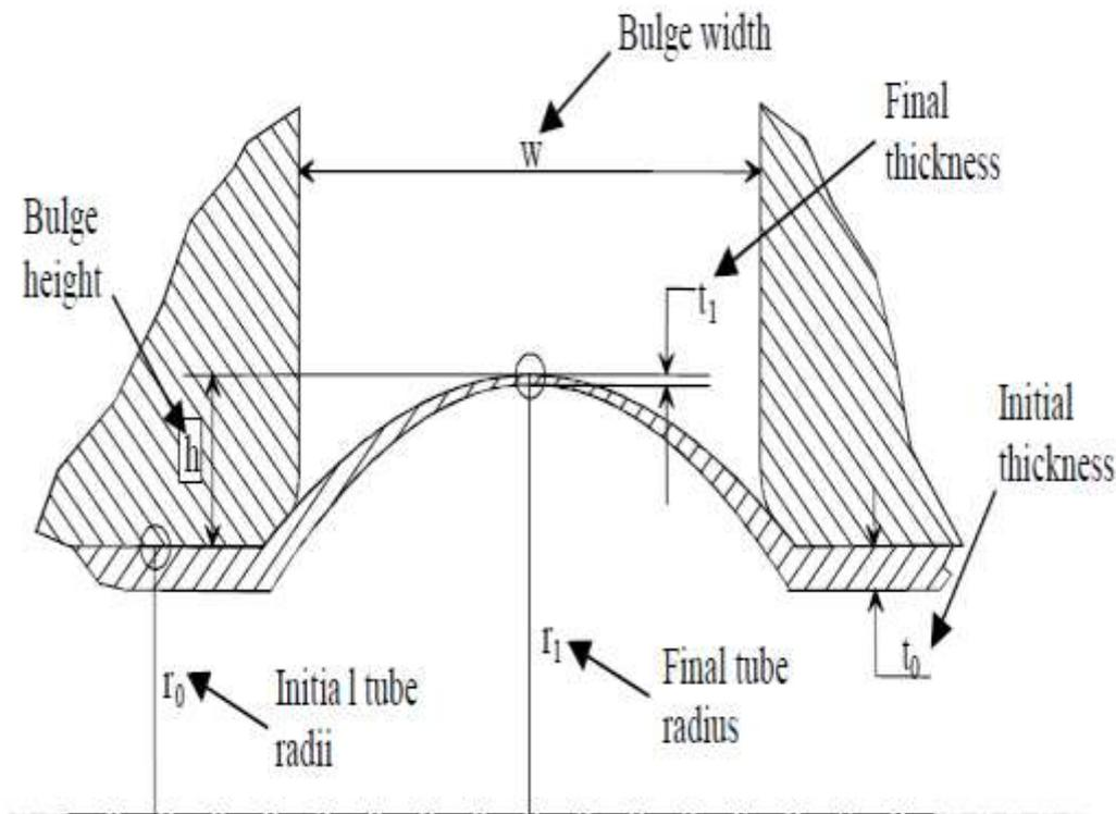
Figure(1) Geometry of the deformed tube.
