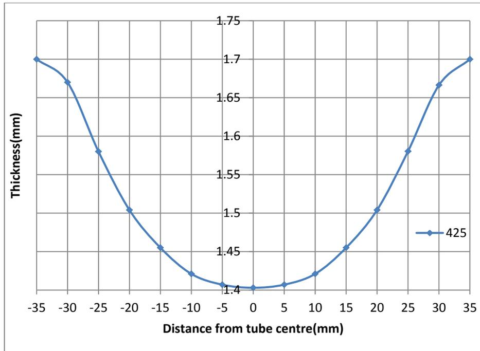
Figure(8) Numerical Thickness distribution.
