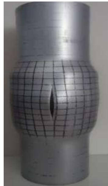
Figure (10) Wrinkling at 7mm axial feeding.
