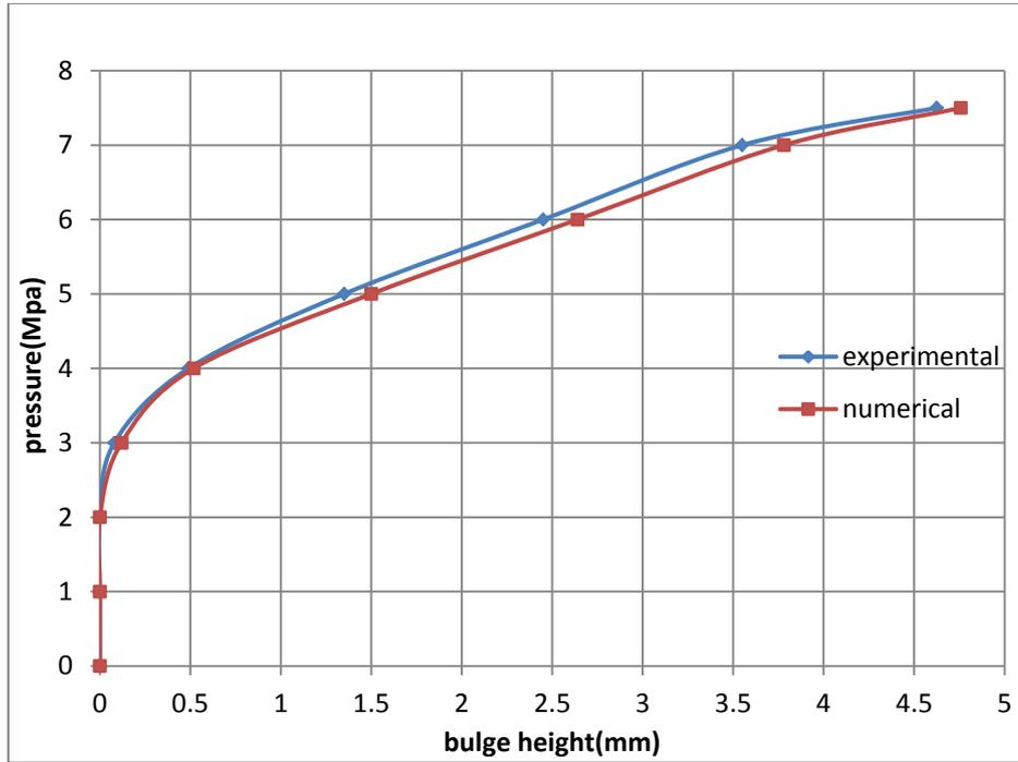
Figure (X) Relationship between pressure and bulge height for tube annealing at 425°C
