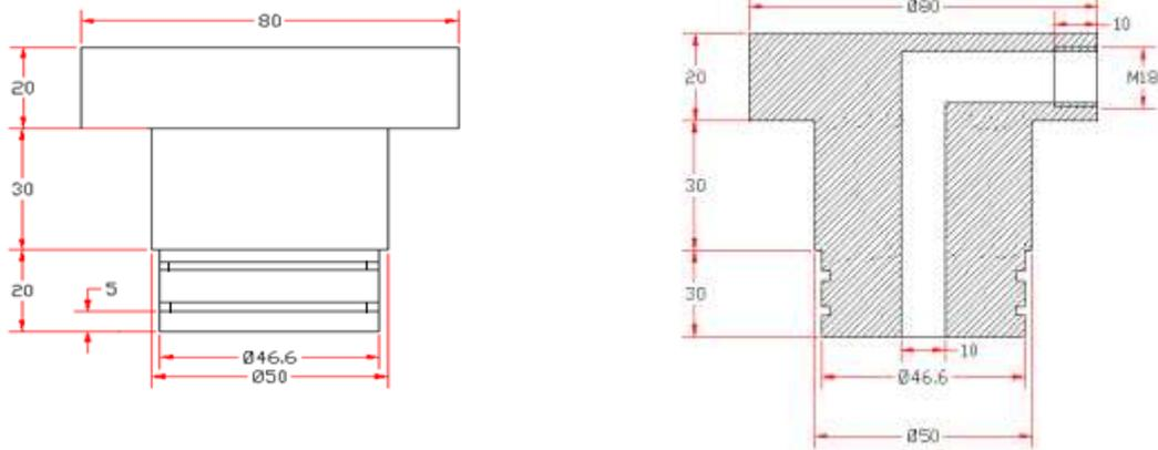
Figure(3) Solid and Hollow punches.
