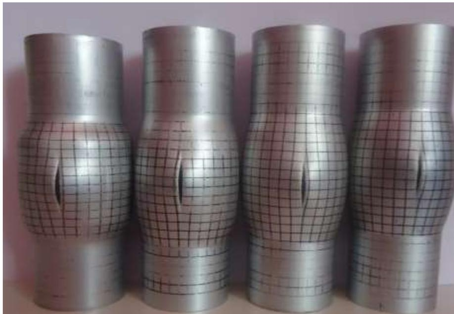
Figure (11) Bulge test at different axial feeding.
