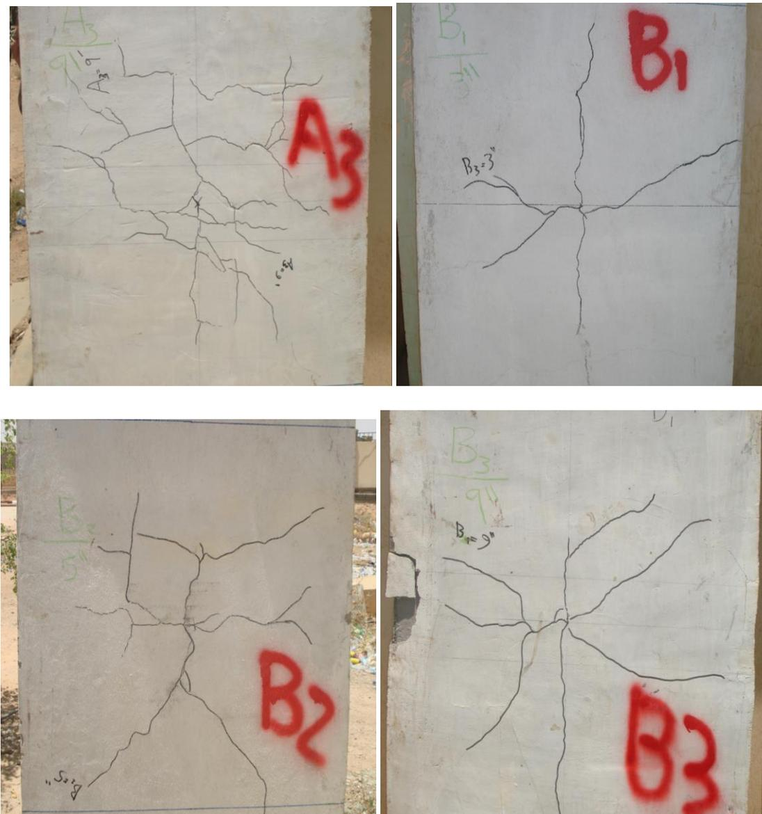
**Fig. (4) Crack pattern for Monopanel slab specimens**
