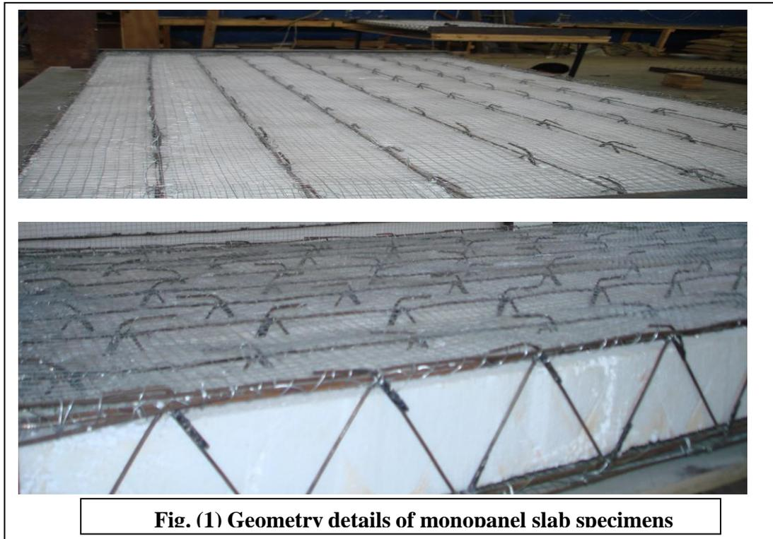
**Fig. (1) Geomtrv details of monopanel slab specimens**
