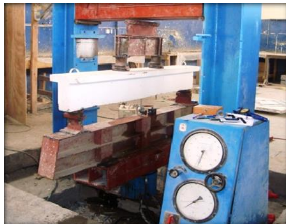
Figure 6: Test set-up of beam specimen
