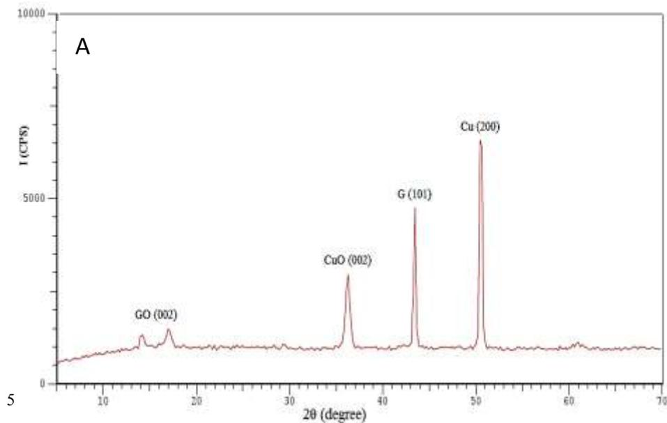
Figure (1): XRD spectrum of multi-layer graphene synthesized at 600<sup>o</sup> C.
