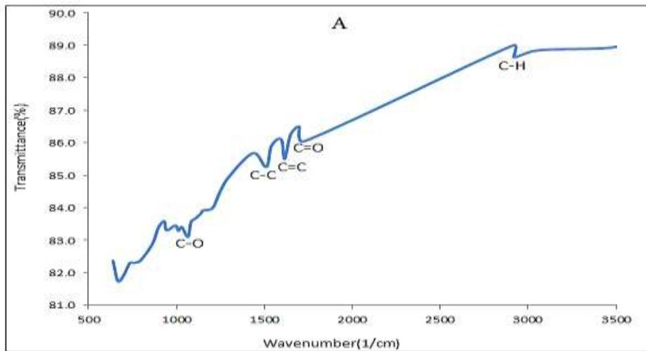
Figure (3): FTIR spectrum of MLG synthesized on Cu at  $600^{\circ}\text{C}$ .
