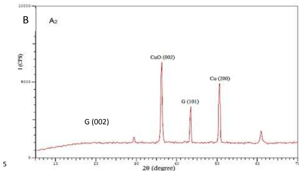
Figure (2): XRD spectrum of multi-layer graphene synthesized at 700<sup>o</sup> C.
