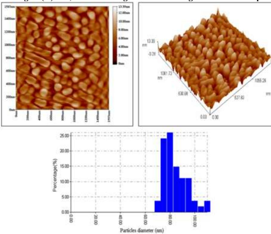
Figure (6): 3D, 2D AFM images and the average size of MLG deposited at 700<sup>0</sup> C.
