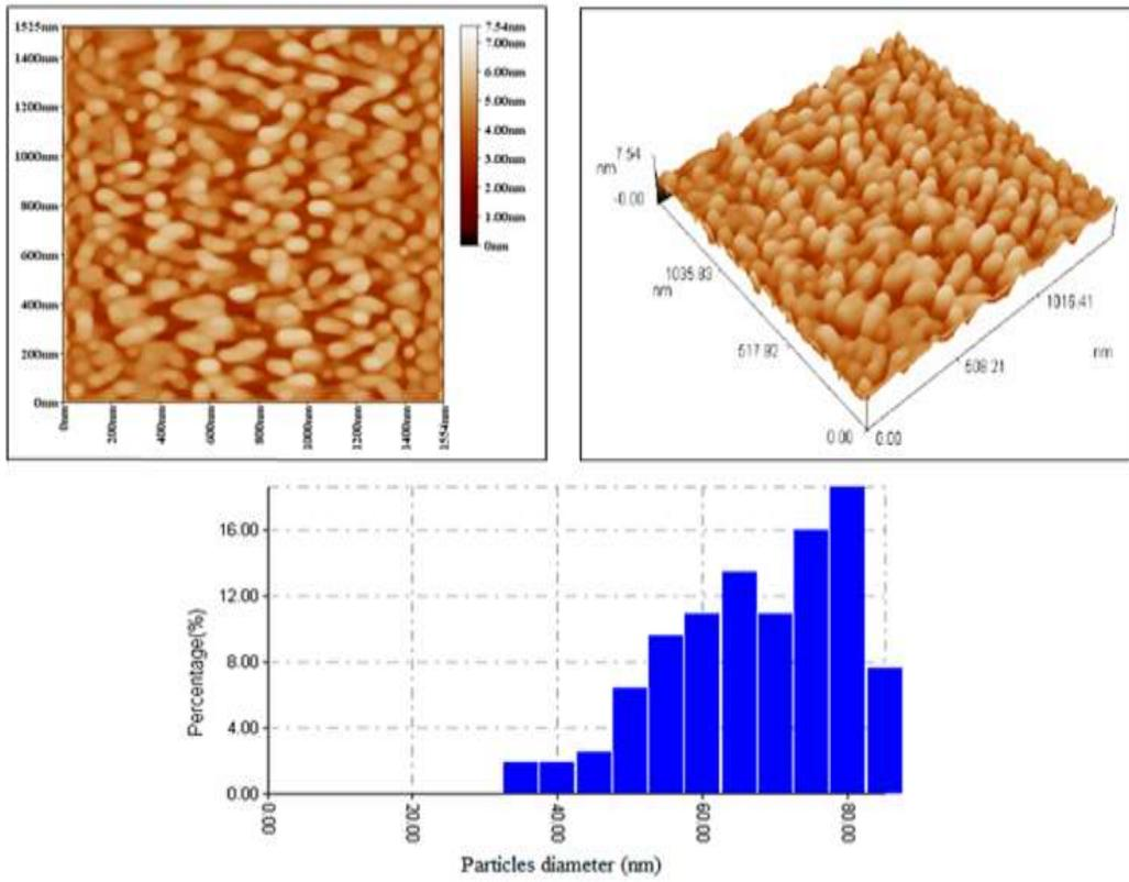
Figure( 5): 3D, 2D AFM images and the average size of MLG deposited at 600<sup>0</sup> C.
