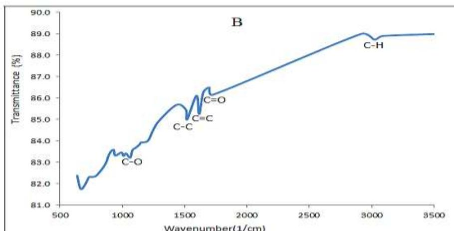
Figure (4): FTIR spectrum of MLG synthesized on Cu at  $700^{\circ}\text{C}$ .
