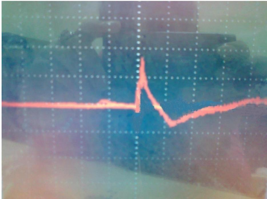
**Figure (15):** Voltage waveform resulting experimentally at 400mJ pulse energy.
