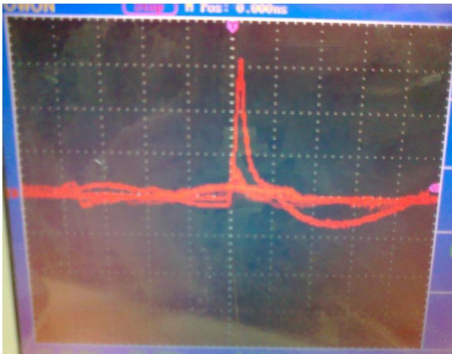
**Figure (11):** Voltage waveform resulting experimentally at 250mJ pulse energy.
