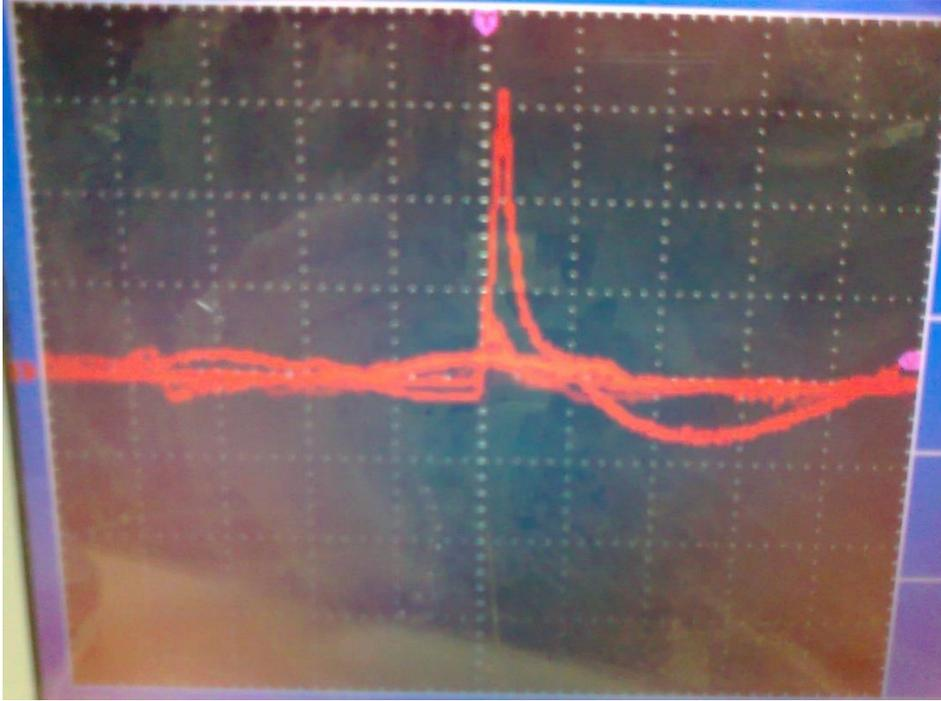
**Figure (12):** Voltage waveform resulting experimentally at 500mJ pulse energy.
