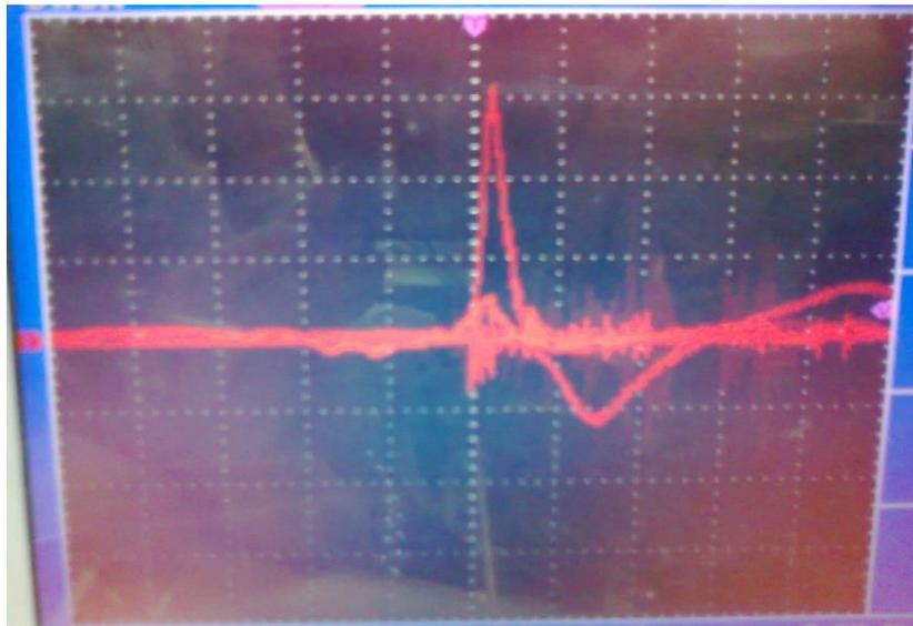
**Figure (7):** Voltage waveform resulting experimentally at 400mJ pulse energy of phantom no1.
