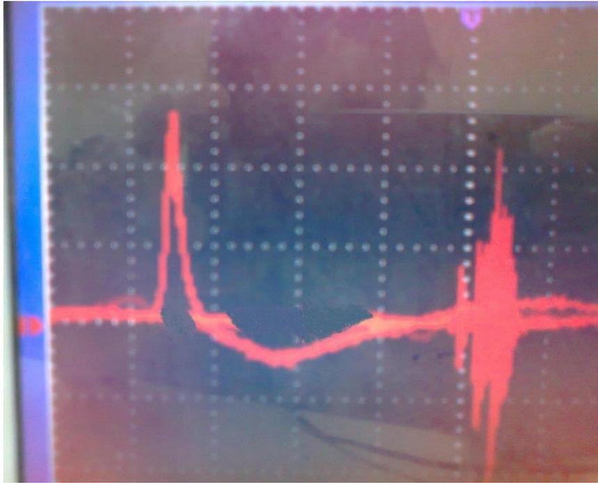
**Figure (18):** Voltage waveform resulting experimentally at 400mJ pulse energy.
