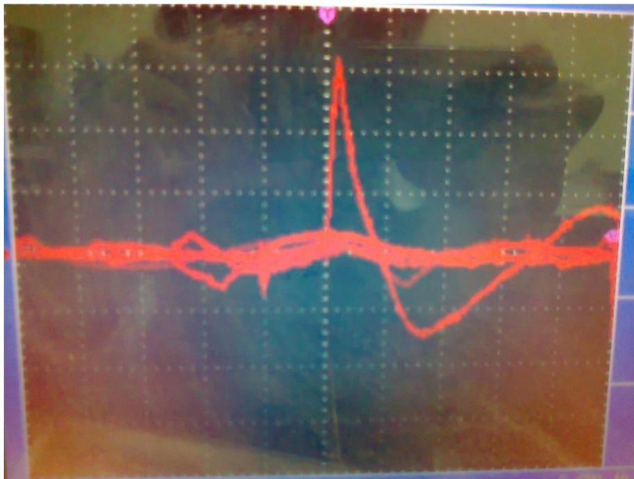
**Figure (19):** Voltage waveform resulting experimentally at 500 mJ pulse energy.
