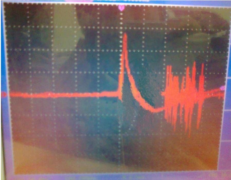
**Figure (20):** Voltage waveform resulting experimentally at 400mJ pulse energy.
