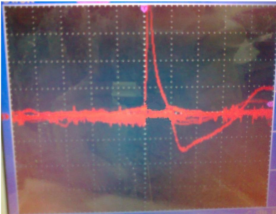
**Figure (9):** Voltage waveform resulting experimentally at 500mJ pulse energy of phantom no.2.
