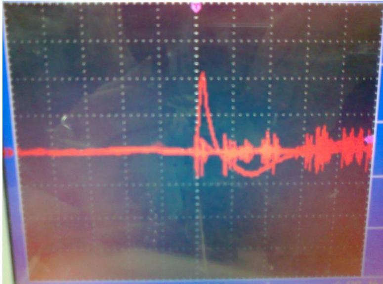
**Figure (8):** Voltage waveform resulting experimentally at 250mJ pulse energy of phantom no.1.
