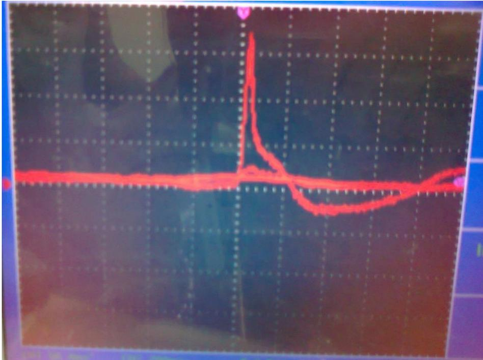
**Figure (10):** Voltage waveform resulting experimentally at 400mJ pulse energy.
