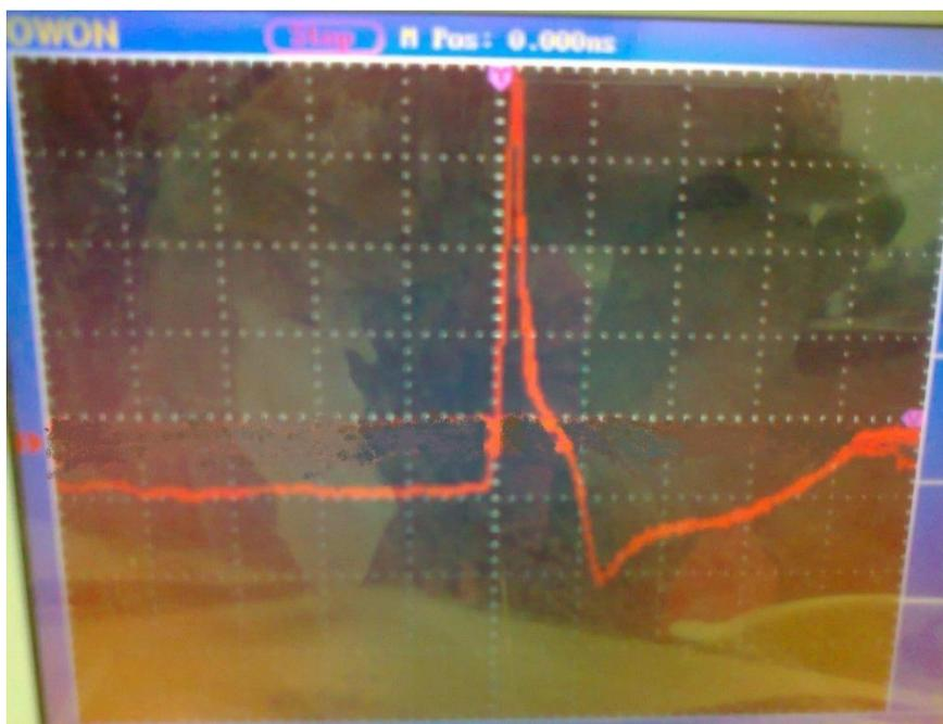
**Figure (17):** Voltage waveform resulting experimentally at 500mJ pulse energy.
