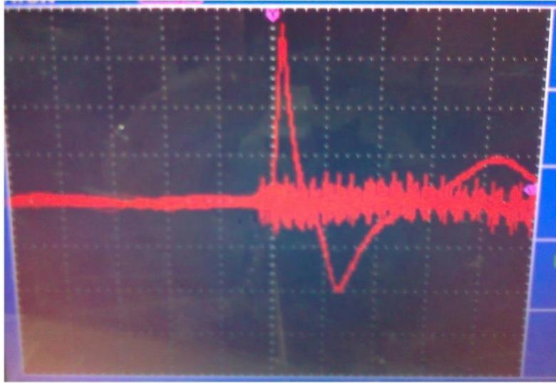
**Figure (6):** Voltage waveform resulting experimentally at 500mJ pulse energy of phantom no.1.
