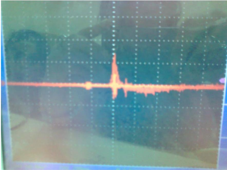
**Figure (16):** Voltage waveform resulting experimentally at 250mJ pulse energy.
