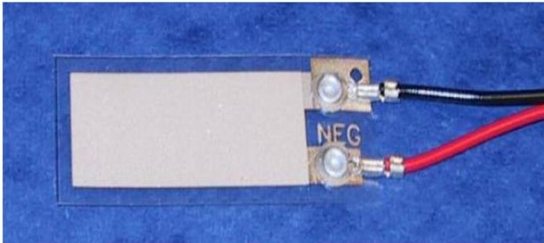
**Figure (4):** Piezoelectric Sensor (LDT1-028K) with lead attachment.
