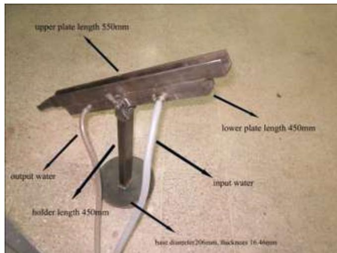
**Figure (2) The instrument of oblique cooling slope.**
